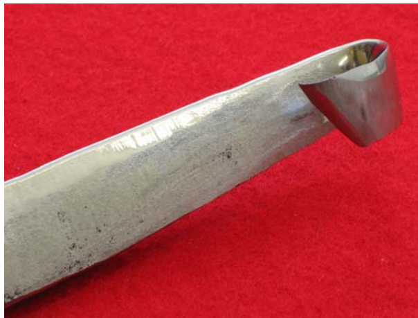
Fig. 2. The cutting tool after 100 hours of service
