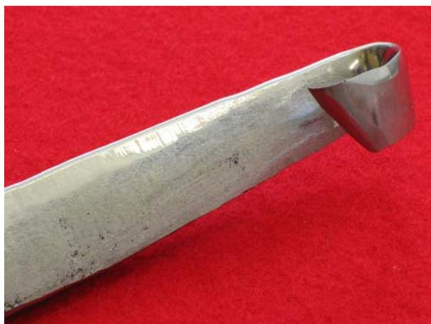
Fig. 2. The cutting tool after 100 hours of service
