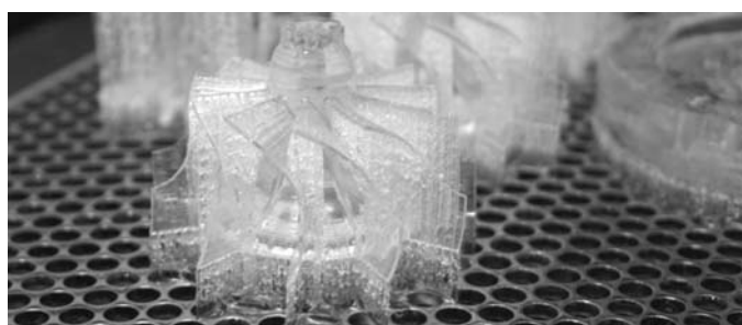
Rys. 5. Stereolitograficzny model wirnika turbiny usytuowany na platformie Fig. 5. Stereolithography model of turbine's rotor on the platform
