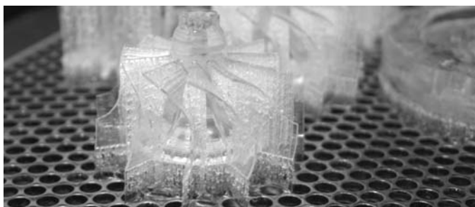
Rys. 5. Stereolitograficzny model wirnika turbiny usytuowany na platformie Fig. 5. Stereolithography model of turbine's rotor on the platform
