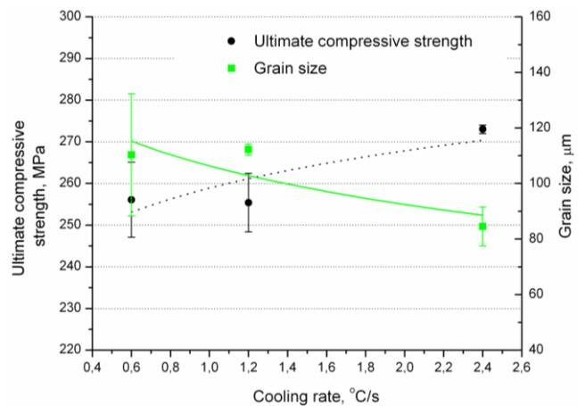
Fig. 6. Variation of the grain size and ultimate compressive strength as a function of cooling rate of analyzed magnesium alloy
