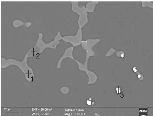
Fig. 3. Representative scanning electron microscope micrograph of magnesium alloy that solidified with cooling rate 0.6°C/s
