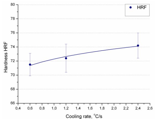
Fig. 7. Variation of the hardness as a function of cooling rate
