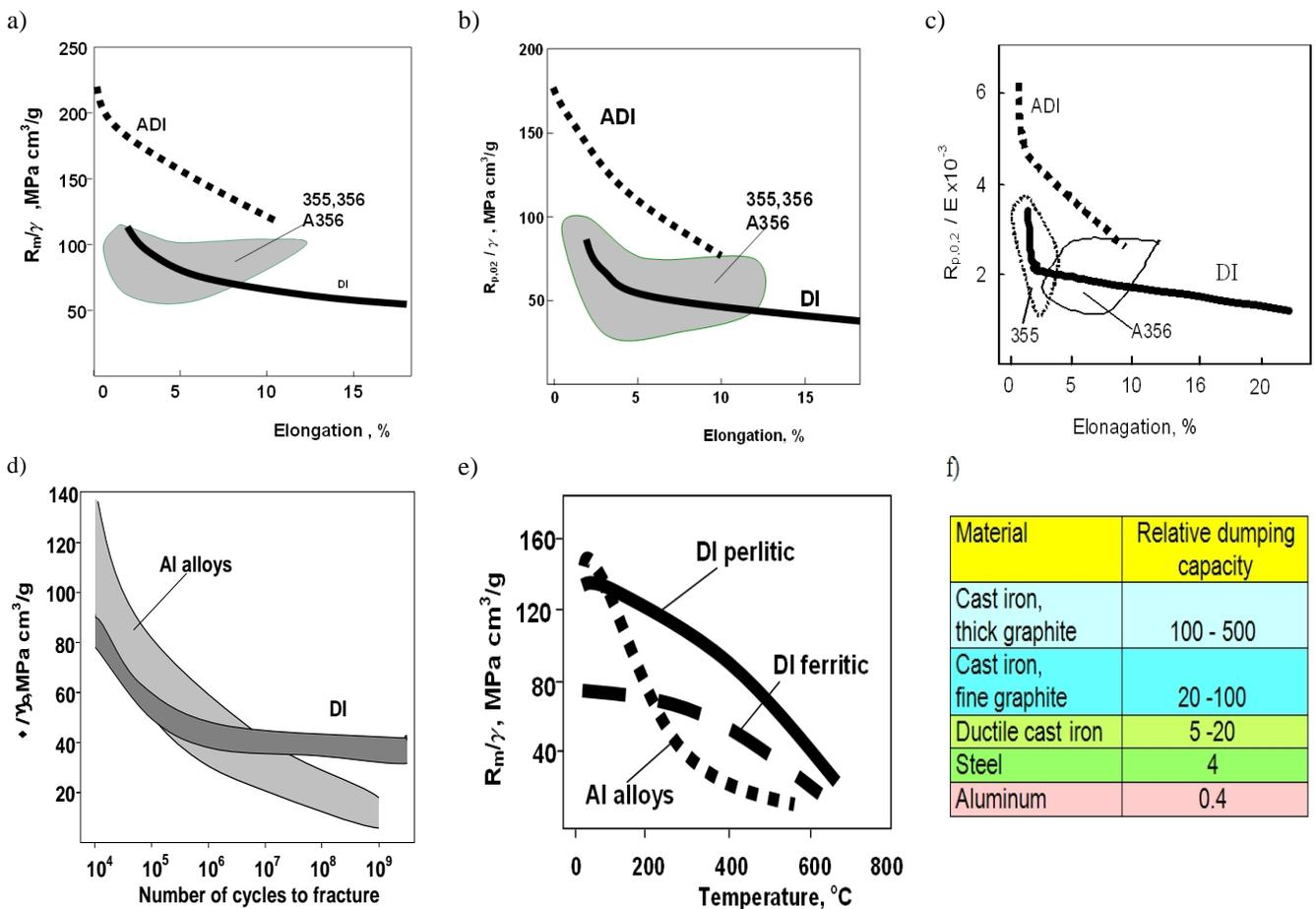
Fig. 1. Relative tensile strength (a,e) yield strength (b) and stiffness indicator (c) fatigue resistance (d) and relative dumping capacity (f); 355, 356, A356 – aluminum alloys. DI – ductile cast iron, ADI – austempered ductile cast iron according to ASTM
