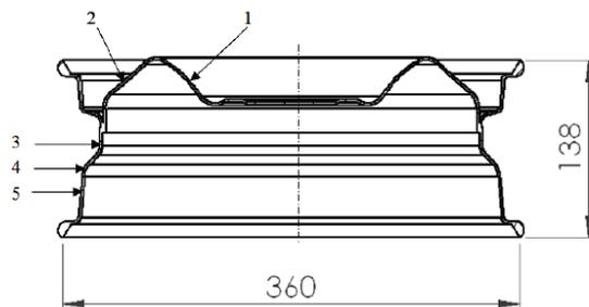
Fig. 9. Cross section of wheel rim made of ductile iron and location of metallographic examinations
