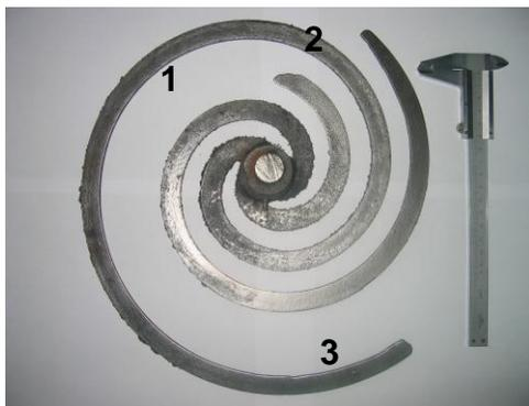
Fig. 5. Photograph of Archimedes spiral and fluidity distance  $L$ ; 1- wall thickness 1 mm,  $L=200$  mm, 2 - wall thickness 2 mm,  $L=650$  mm, 3- wall thickness 3 mm,  $L=1090$  mm
