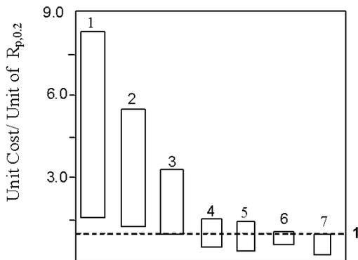
Fig. 2. Unit costs<sup>1</sup> of product essential for obtaining unit yield strength  $R_{p0.2}$  normalized towards forget steel (up to 1); (1) - aluminum alloys castings, (2) – forged aluminum, (3) – cast steel, (4) – forged steel, (5) - heat treated steel, (6) – ductile iron, (7) – ADI [1]
