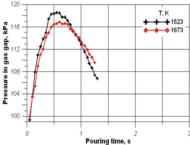
Fig. 10. Gas pressures measured in the gas gap for different temperatures when poured with cast iron
