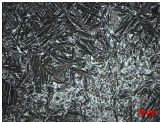
Fig. 5. Microstructure of ADI from C2 cycle. Etched with Beraha reagent - Martensite, 1000x. Pre-eutectoid ferrite, lower bainite, austenite
