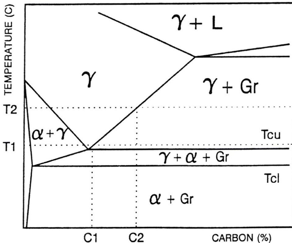
Fig. 1. Qualitative 2 D image of the phase equilibrium diagram for a ternary Fe-C-Si system containing 2,5% Si.  $\gamma$  – austenite,  $\alpha$  – ferrite, G – graphite,  $T_{cu}$  – upper critical austenitising temperature,  $T_{cl}$  – lower critical austenitising temperature [4]
