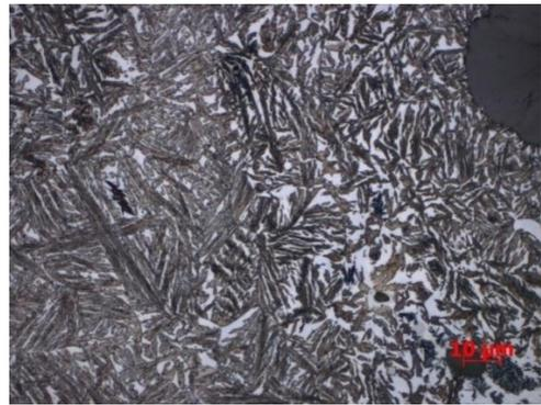
Fig. 9. Microstructure of ADI from C6 cycle. Etched with Beraha reagent - Martensite, 1000x. Pre-eutectoid ferrite, lower bainite, austenite
