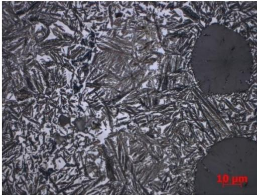
Fig. 6. Microstructure of ADI from C3 cycle. Etched with Beraha reagent - Martensite, 1000x. Pre-eutectoid ferrite, lower bainite, austenite
