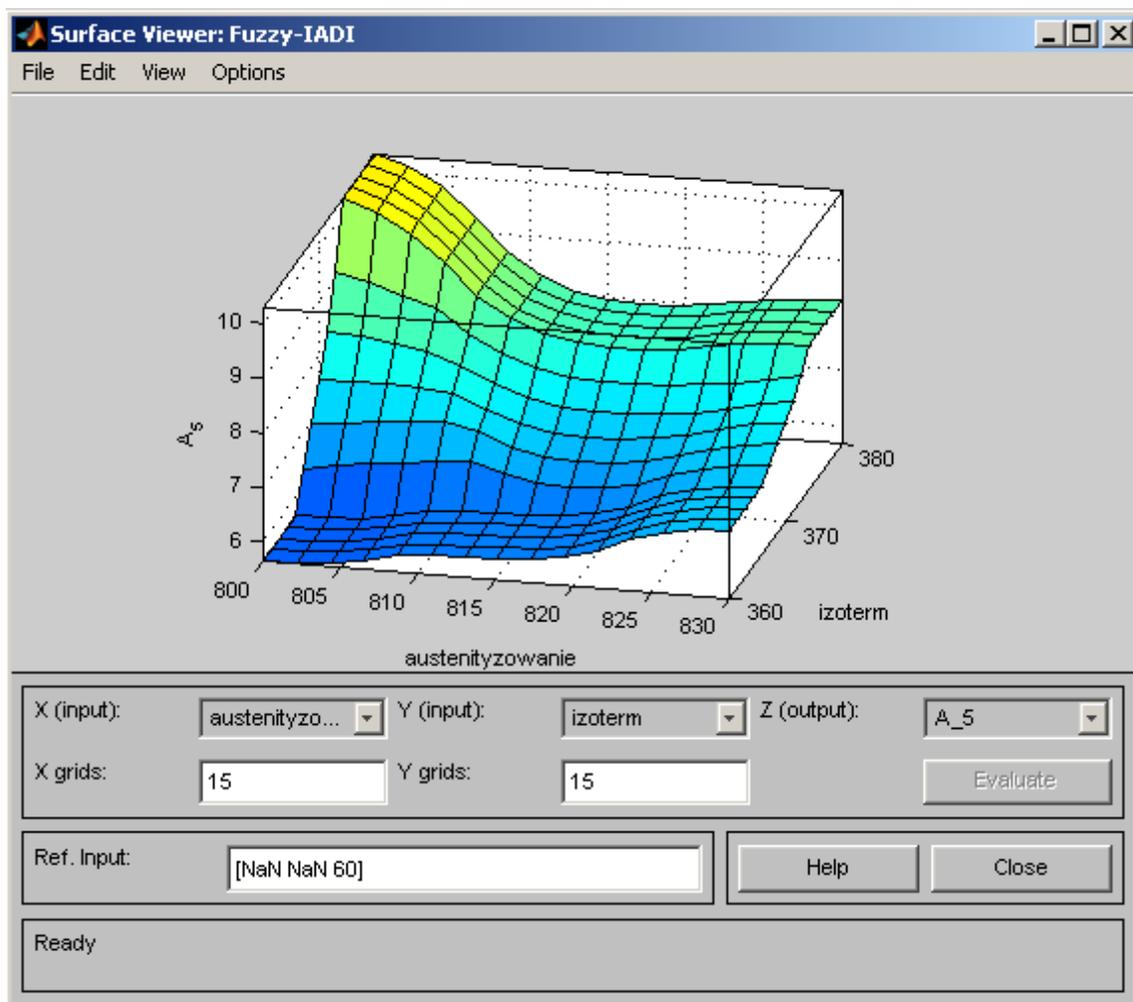
Fig. 14. Relationship between the elongation EL and heat treatment conditions
