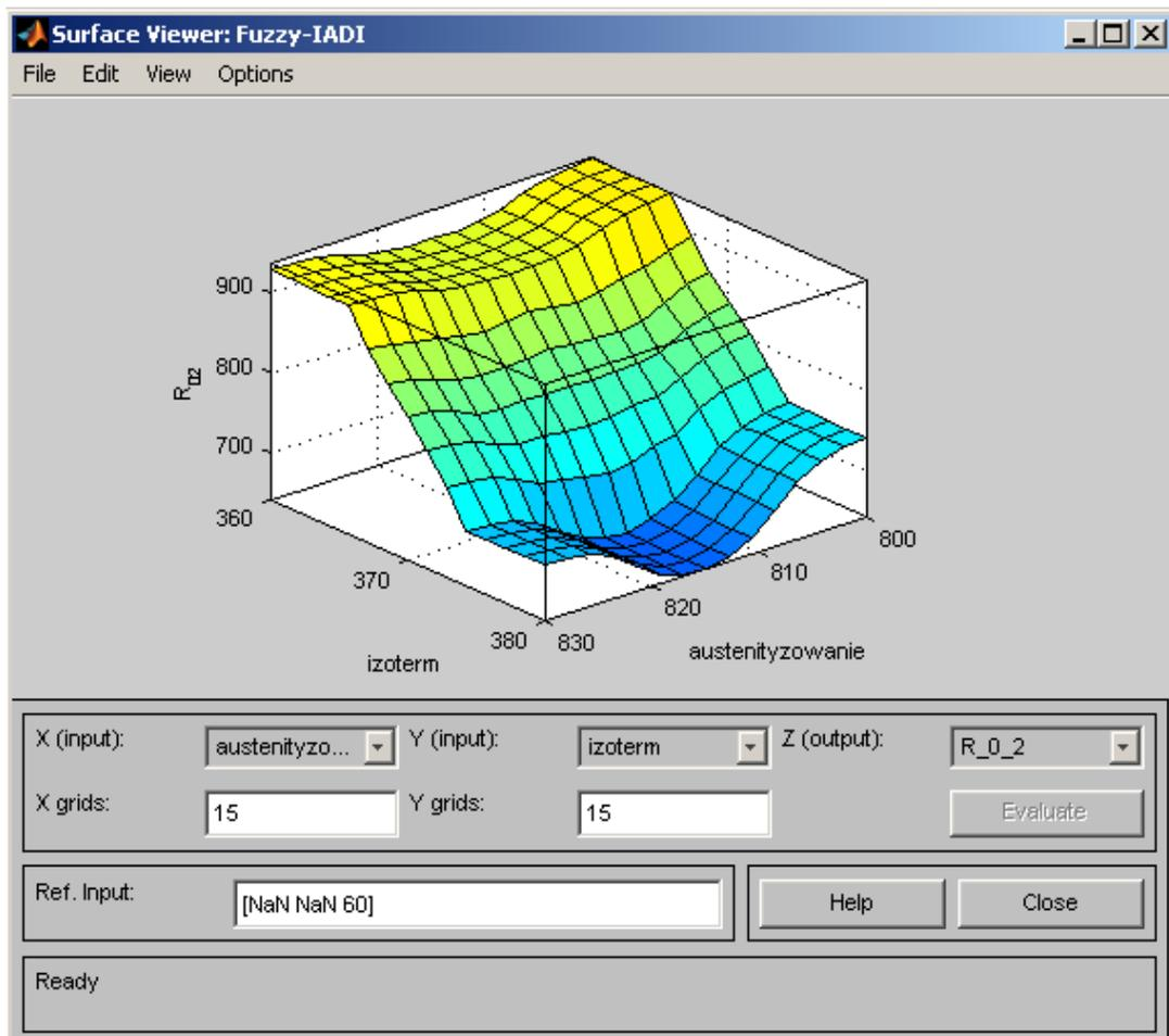
Fig. 13. Relationship between the yeild strength YS and heat treatment conditions
