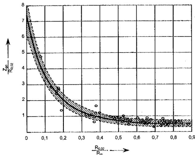
Fig. 1. Curve used in fatigue strength assessment [15]
