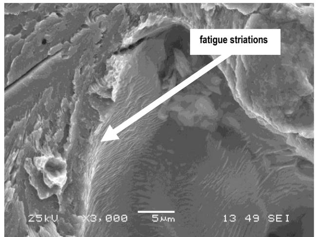
Ductile iron. Specimen 3, x3000, SEM.
