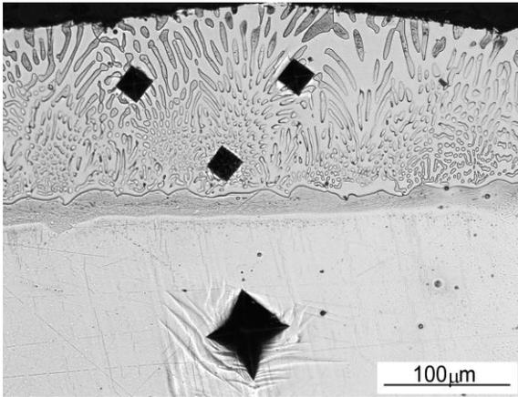
Fig. 3. Microhardness measurement indentations in the Al-enriched layer and the Mg substrate
