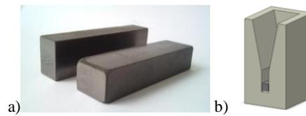
Fig. 1. Packets for the carbide synthesis (a) and 3D drawing of the mould cross-section with packet placed at the bottom (b)
