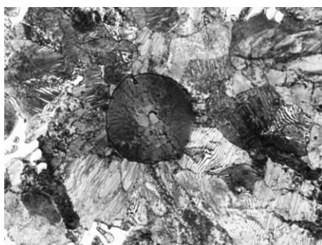
a) Microstructure: nodular graphite, pearlite, carbides, non-metallic inclusions
