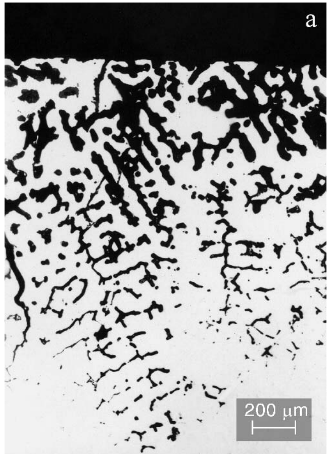
Fig. 5. Impact sample scraps in commercial melts Cr–Ni cast steel of 18/8 + Ti type. Heat treatment: solution heat treatment + stabilization: a – melts without modification, 0.62%Ti, 6.5% Fe – δ, b – melts modified with cerium mixture, 0.51%Ti, 7.0% Feδ
