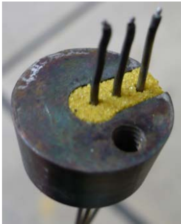
Fig. 2. Closing conical insert (No. 22' in Fig. 1.) with embedded thermocouples
