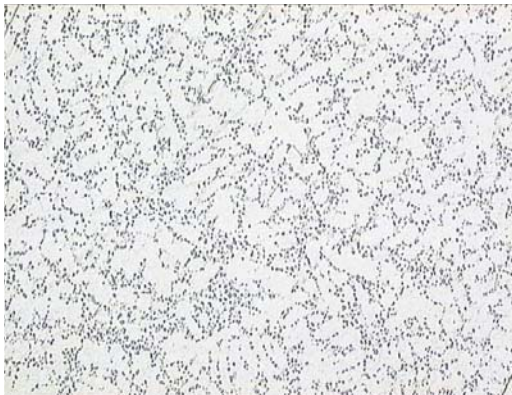
Fig. 4. Microstructure of AK9 alloy after dispersion hardening, magnification 300x
