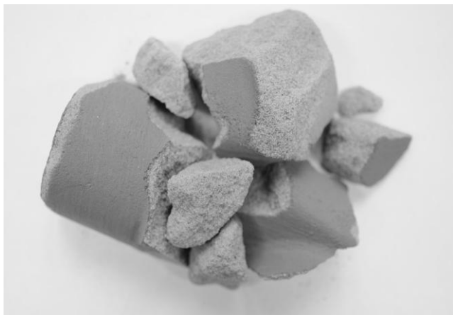
Fig. 4. View of waste moulds and cores before utilization in the microwave chamber; moulding sand M1
