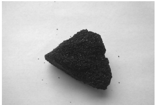
Fig. 5. View of waste moulds and cores before utilization in the microwave chamber; moulding sand M2
