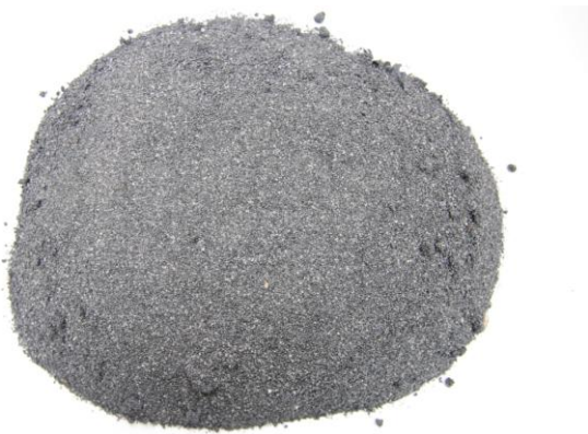
Fig. 7. View of moulds and cores completely incinerated in microwave chamber; moulding sand M2
