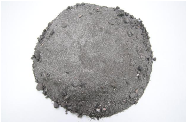
Fig. 6. View of moulds and cores completely incinerated in microwave chamber; moulding sand M1
