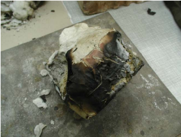
Fig. 5. The view of burnt through sample after cooling before cutting and grinding down
