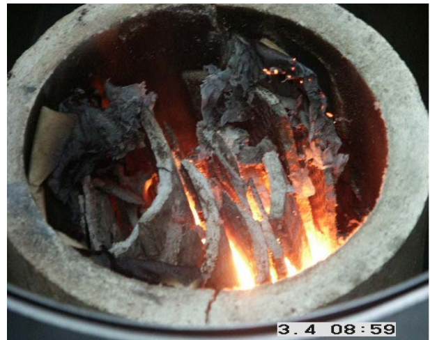
Fig. 3. The view of the interior of the microwave reactor's chamber after the short-lived batch heating - visible pieces of plates of the asbestos-cement roofing material
