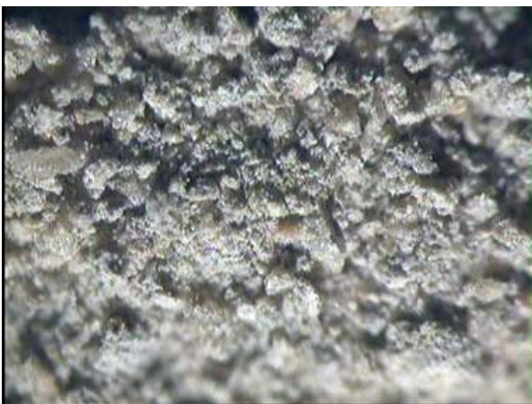
Fig.7. Asbestos-cement roofing material neutralized in the microwave reactor with the 1:1 participation of the X substance. Light microscope; enlarging 25:1
