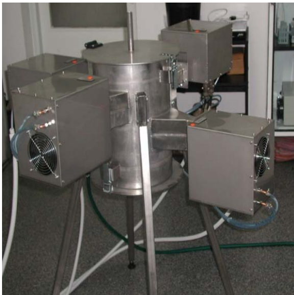
Fig. 2. The view of the reactor chamber with installed generators
