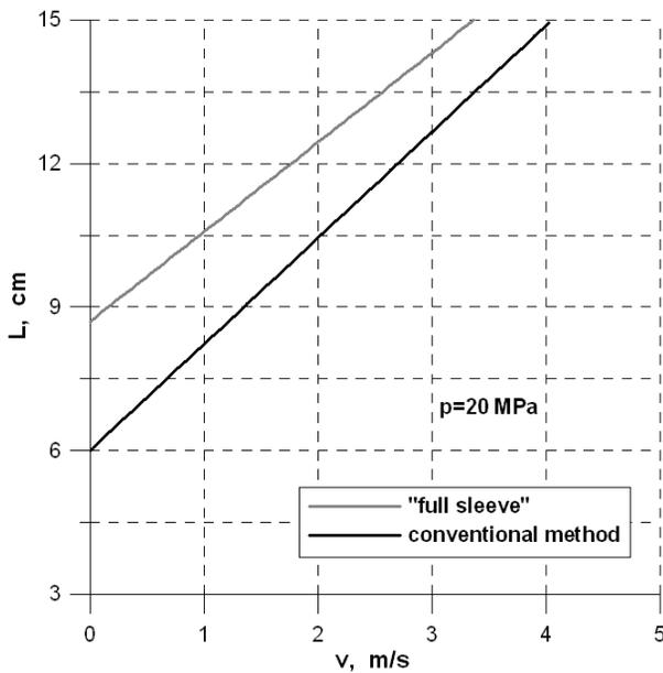
Fig.3. Dependence of alloy castability on the plunger speed in the second phase of injection at the pressure of 20 MPa
