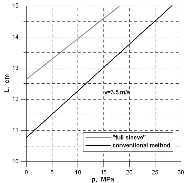
Fig.5. Dependence of alloy castability on the intensification pressure at the plunger speed equal to 3.5 m/s
