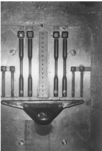
Fig.2. Pressure die with an insert for the castability test
