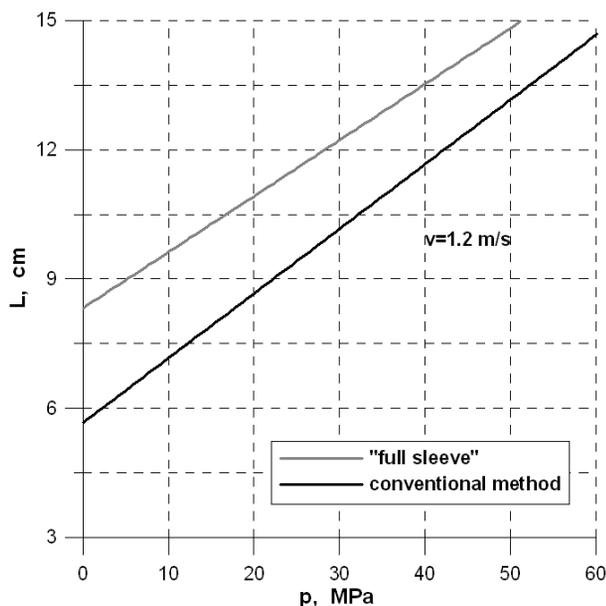
Fig.6. Dependence of alloy castability on the intensification pressure at the plunger speed equal to 1.2 m/s
