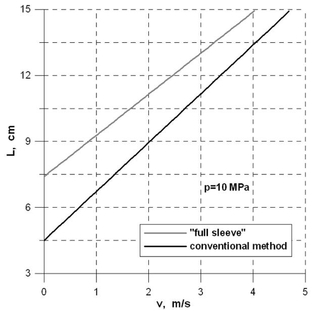
Fig.4. Dependence of alloy castability on the plunger speed in the second phase of injection at the pressure of 10 MPa
