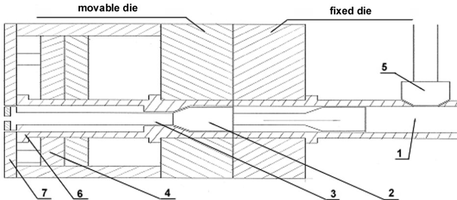
Fig.1. 'Full sleeve' construction with a counter plunger; 1-shot sleeve, 2-counter plunger, 3-counter plunger rod, 4-ejector plate, 5- stopper closing the shot sleeve, 6-sleeve, 7- mounting plate.
