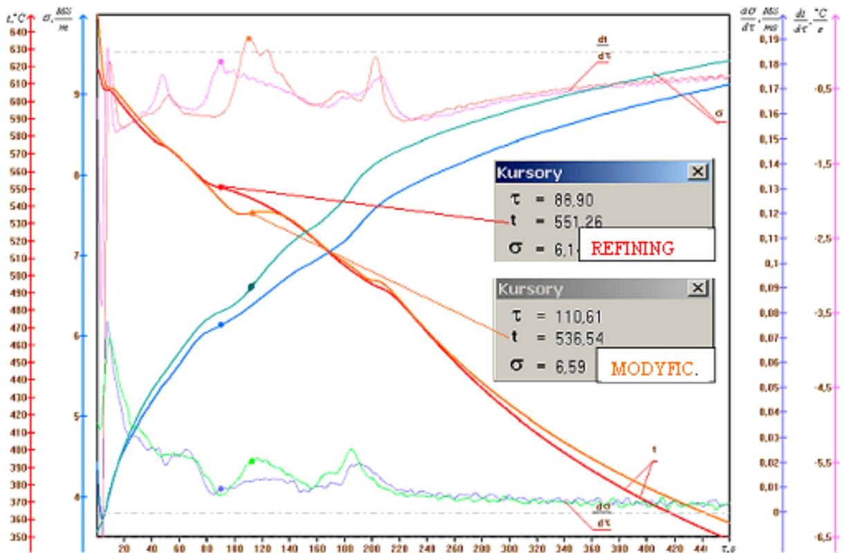
Fig. 1. Crystallization curves for the alloy AK64 cast into the ceramic moulds
