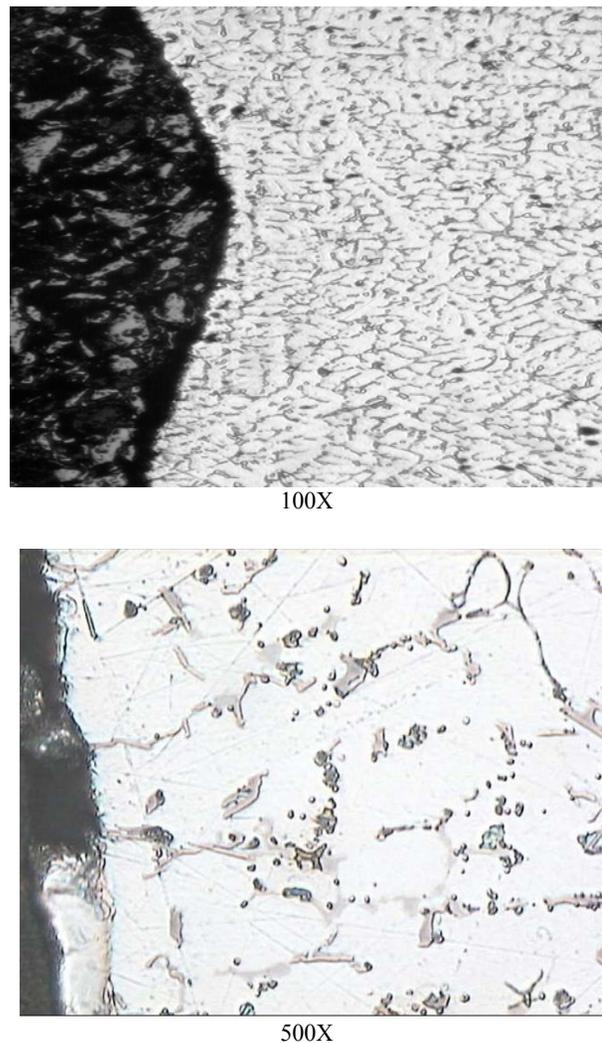
Fig. 4. Shapes and distribution of the retained impurities in the ceramic filter cast with the alloy studied
