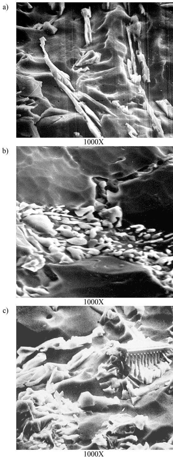
Fig. 3. Microstructures of the upgraded alloy AK64 cast into the ceramic moulds: a – refined alloy, b – modified alloy, c – view of secondary phases
