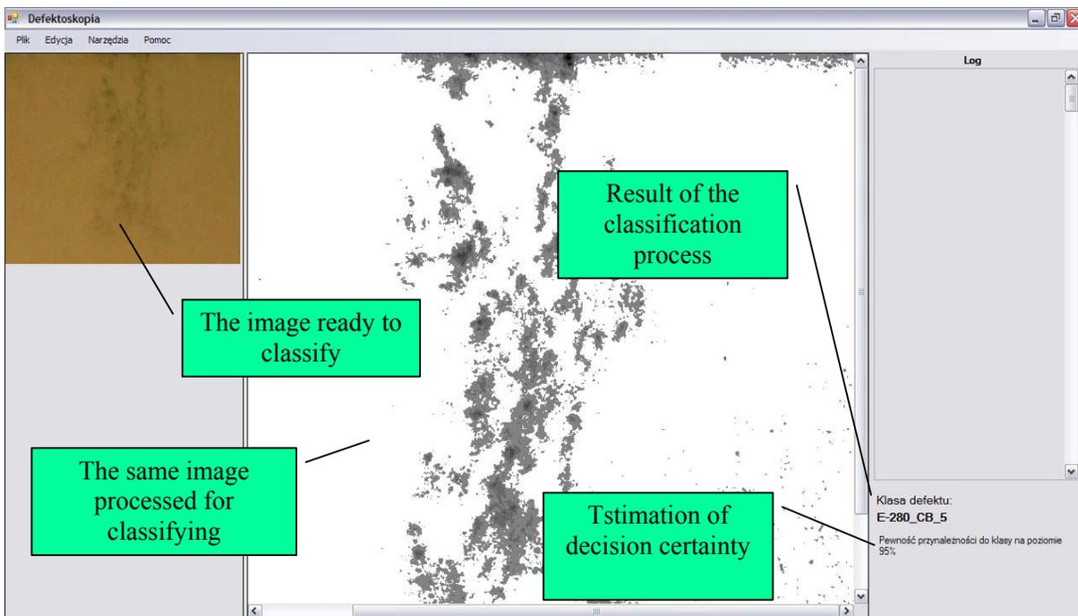
Fig 7. Result of the classifying process
