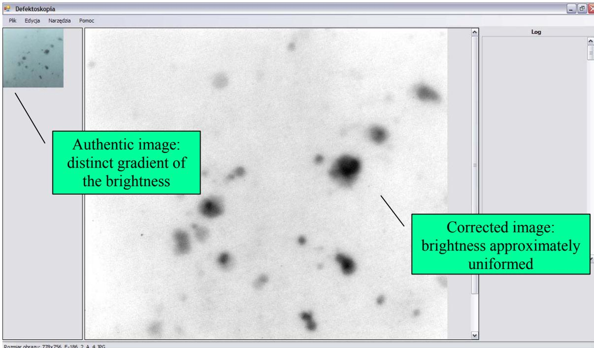
Fig.3 Model result of lighting unevenness correction.
