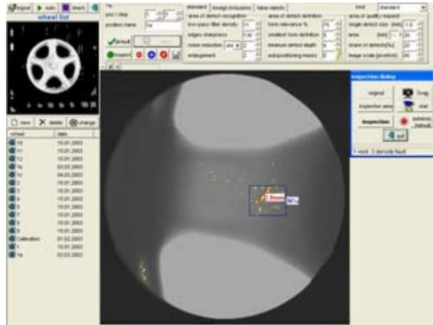
Fig. 1 Identification of casting defects in the Xpect program [14]
