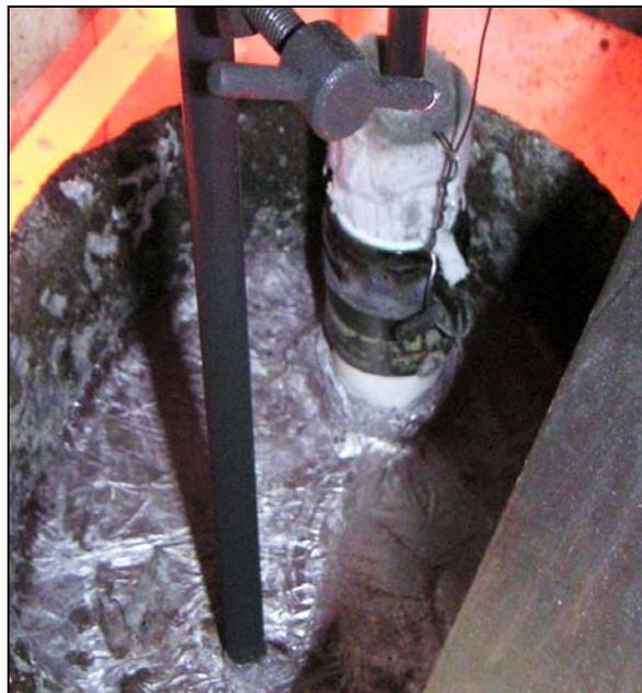
Fig. 5. General view of the test stand. A retort made from "beta-alumina" immersed in liquid alloy.
