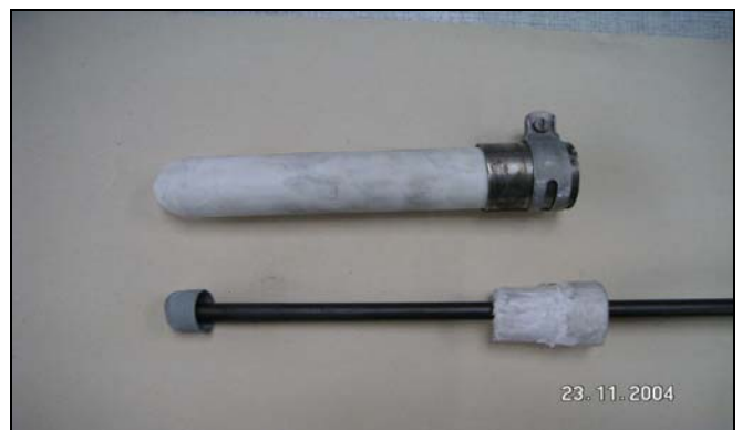
Fig.3. "Beta alumina" retort blind-closed on one end, provided with fixing elements and ready for the experiment. Graphite electrode with elements stabilizing its location.
