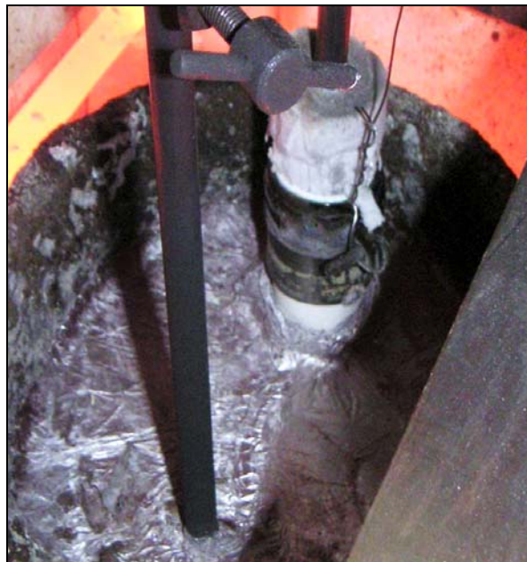
Fig. 5. General view of the test stand. A retort made from "beta-alumina" immersed in liquid alloy.
