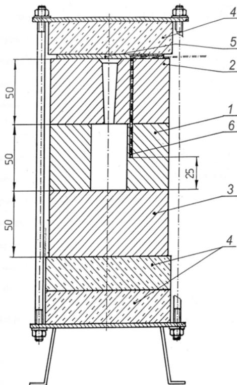
Fig. 2. Test mould: 1 – test shape (mould), 2 – upper insulating shape, 3 – lower insulating shape, 4 – insulating disc, 5 – aluminosilicate paper, 6 – thermocouple.
