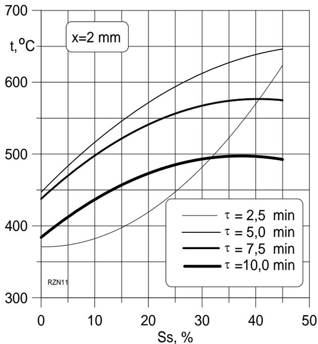
Fig. 7. Dependence of temperature of a mould of foamed plaster on the degree of foaming  $S_s$  for:  $\tau = 2,5; 5,0; 7,5$  and  $10,0$  min and  $x = 2$  mm.
