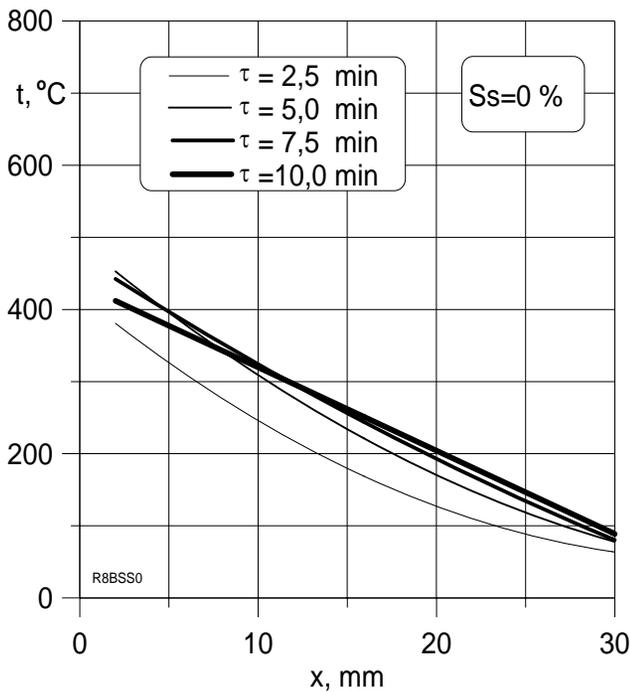
Fig. 6. Dependence of temperature of plaster mould  $t$  on the distance  $x$  for:  $\tau = 2,5; 5,0; 7,5$  and  $10,0$  min and  $S_s = 0\%$ .
