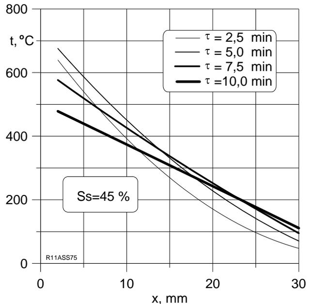
Fig. 5. Dependence of temperature of a mould of foamed plaster  $t$  on the distance  $x$  for:  $\tau = 2,5; 5,0; 7,5$  and  $10,0$  min and  $S_s = 45\%$ .
