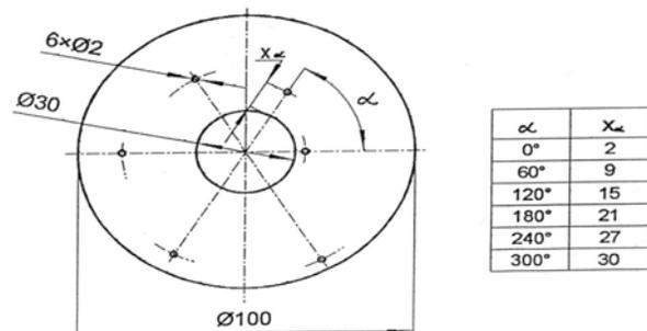
Fig.1. Scheme of spacing the holes for thermocouples in the test mould.
