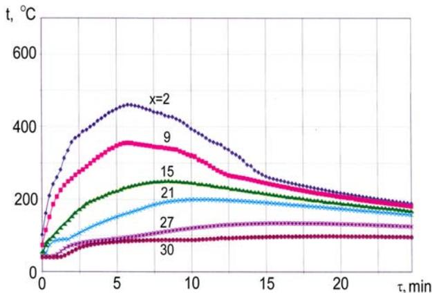
Fig. 4. Dependence of temperature of plaster mould on the cast cooling time  $\tau$  for:  $x=2, 9, 15, 21, 27$  and  $30$  mm and  $S_s=0\%$
