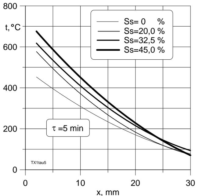
Fig. 8. Dependence of temperature of a mould of foamed plaster on the distance  $x$  for:  $S_s = 0; 20; 32,5$  and  $45\%$  and  $t = 5$  min.
