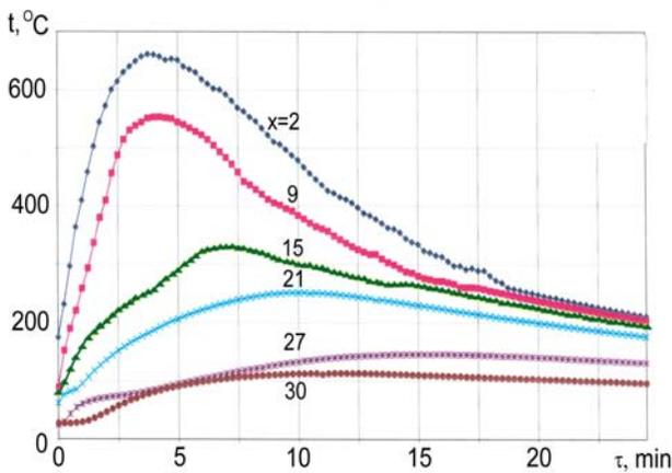
Fig. 3. Dependence of temperature of a mould of foamed plaster on the cast cooling time  $\tau$  for:  $x=2, 6, 15, 27$  and  $30$  mm and  $S_s=45\%$ .
