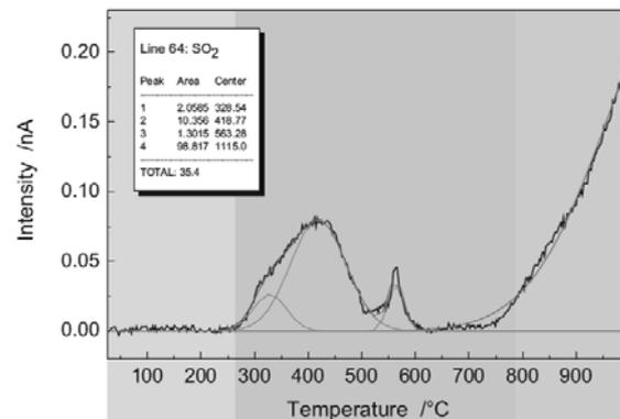
Fig. 5. Range of SO2 emission from a bentonite-carbon mixture
