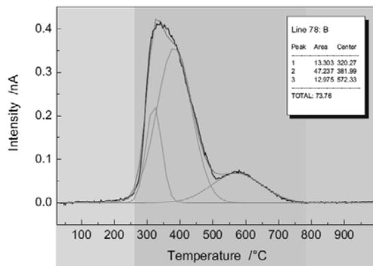
Fig. 7. Range of benzene emission from a bentonite-carbon mixture
