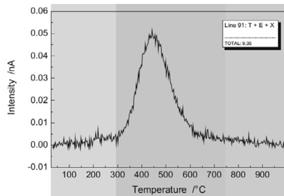
Fig. 10. Range of toluene, ethylbenzene and xylenes emission from a dust
