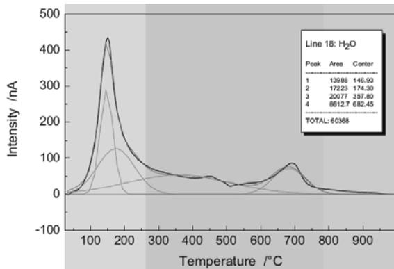
Fig. 1. Range of water emission from a bentonite-carbon mixture
