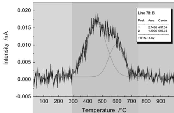
Fig. 8. Range of benzene emission from a dust
