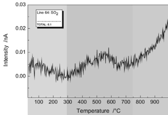
Fig. 6. Range of SO<sub>2</sub> emission from a dust
