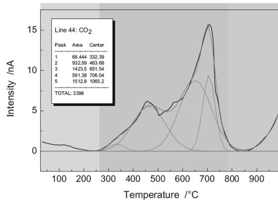
Fig. 3. Range of CO2 emission from a bentonite-carbon mixture
