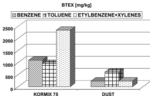
Fig. 13. BTEX emission from the bentonite-carbon mixture and from dusts
