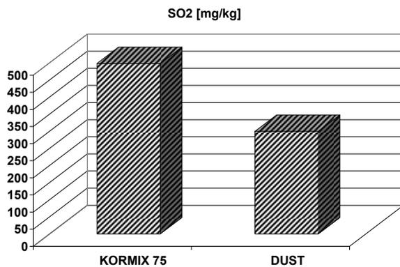
Fig. 12. SO<sub>2</sub> emission from the bentonite-carbon mixture and from dusts
