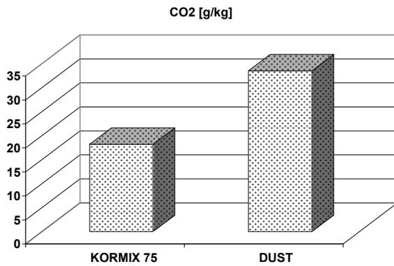
Fig. 11. CO<sub>2</sub> emission from the bentonite-carbon mixture and from dusts
