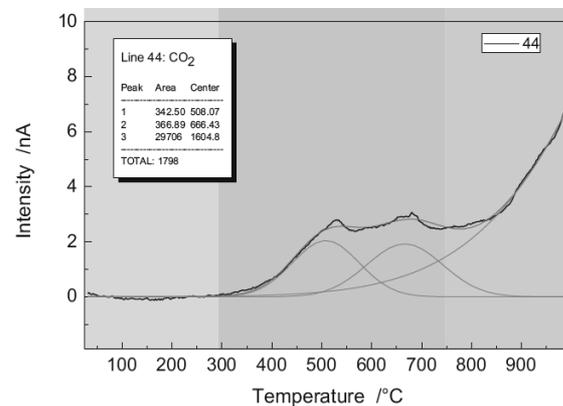
Fig. 4. Range of CO2 emission from a dust
