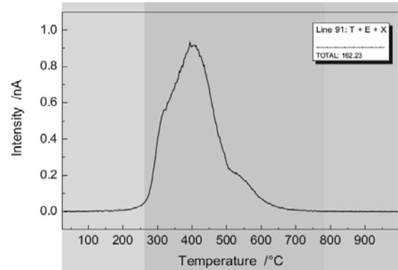
Fig. 9. Range of toluene, ethylbenzene and xylenes emission from a bentonite-carbon mixture
