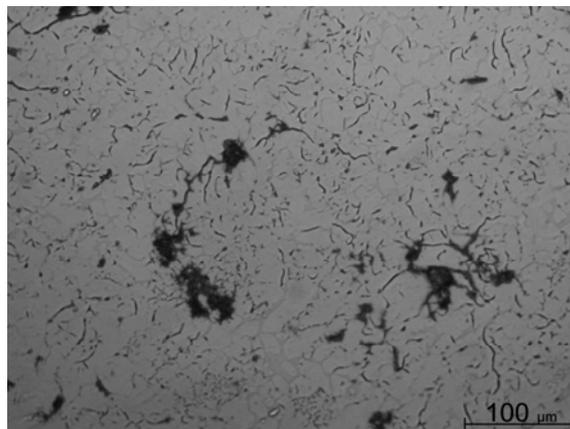
Fig.2. Microstructure of grey cast iron EN-GJL-200 after cast to graphite mould
