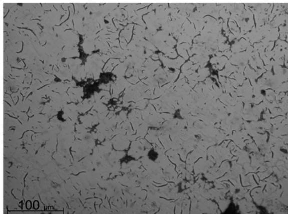
Fig.5. Microstructure of grey cast iron EN-GJL-200 after cast to graphite mould with influence of rotate electromagnetic field
