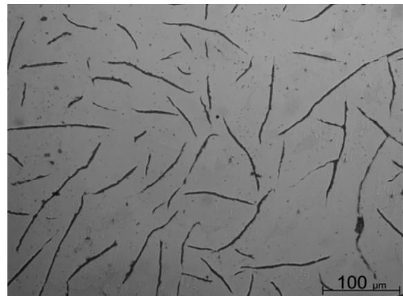
Fig.7. Microstructure of grey cast iron EN-GJL-200 after cast to Sibral mould with influence of rotate electromagnetic field
