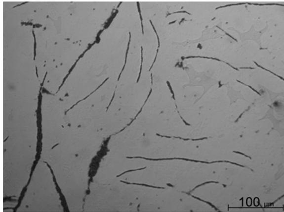
Fig.4. Microstructure of grey cast iron EN-GJL-200 after cast to Sibral mould
