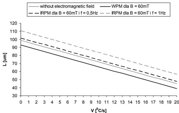
Fig.9. Influence of cooling rate in temperature range  $T_{ZAL} \div T_L$  ( $V$ ) on average length of flake graphite ( $L$ ) in structure of grey cast iron EN-GJL-200 for casting without and with influence of electromagnetic field
