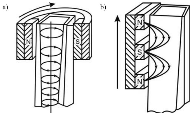
Fig. 1. The scheme of an electromagnetic stirrer enforcing (a) rotary reversion and (b) oscillatory motion of liquid metal along the axis originating ingot [2, 3]
