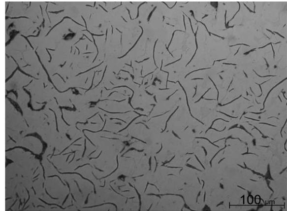
Fig.6. Microstructure of grey cast iron EN-GJL-200 after cast to shell mould with influence of rotate electromagnetic field
