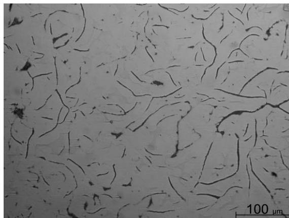
Fig.3. Microstructure of grey cast iron EN-GJL-200 after cast to shell mould
