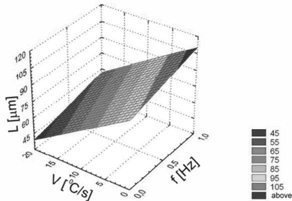
Fig. 8. Average length of flake graphite ( $L$ ) in structure of grey cast iron EN-GJL-200 in function of pulse frequency of electromagnetic field ( $f$ ) and cooling rate ( $V$ ) – for casting with influence of electromagnetic field about value of magnetic induction  $B = 60\text{mT}$
