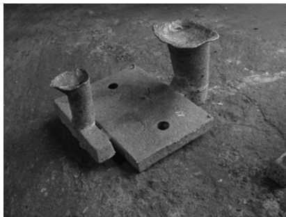
Fig. 1. The appearance of a test casting with the gating system immediately after knocking out from mould
