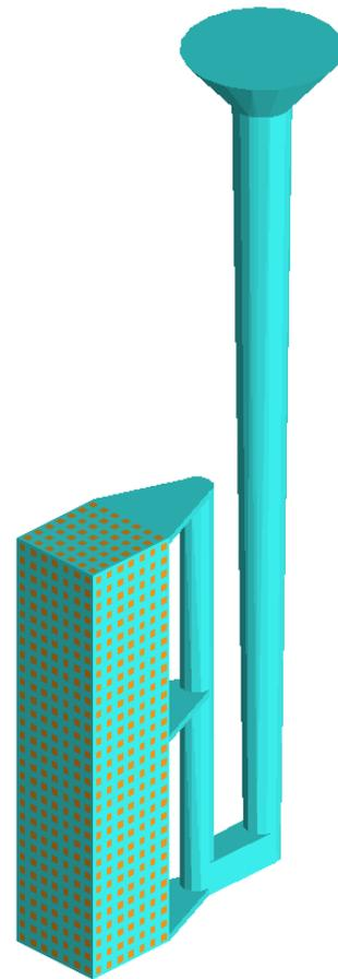
Fig 1. The view of the model cast with its core and multi-level getting system
