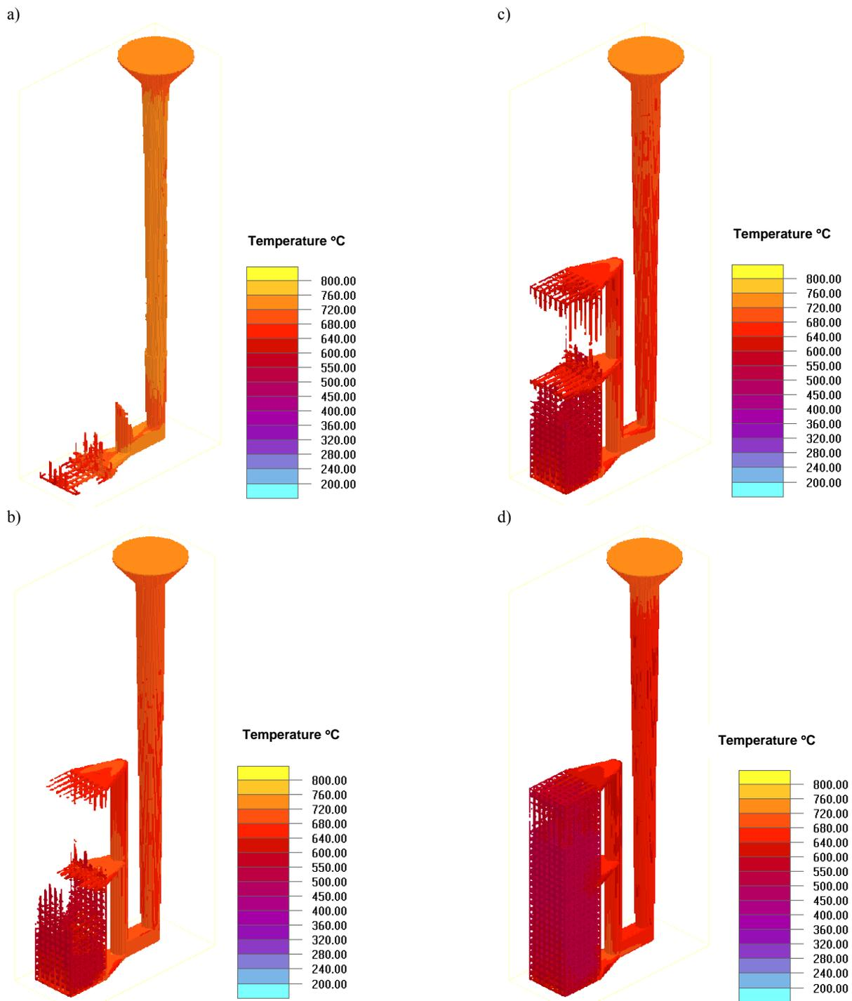
Fig. 2. The results of filling and temperature distribution during casting and cooling the virtual cast. The scale is adequate to the established local temperature of the cast.
