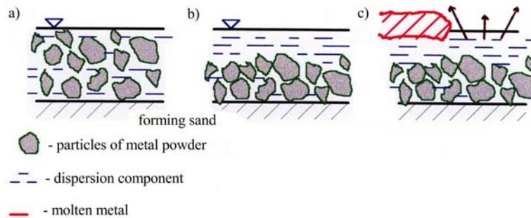
Fig. 2. The mould's coating during casting a) mould's coating after spraying, b) sedimentation of metal particles, c) molten metal pouring
