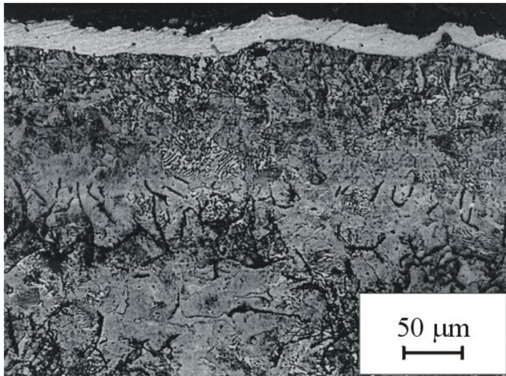
Fig. 4. Structure of casting's surface with two layers of VINAMUL 36/50 coating
