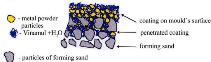
Fig. 1. The created mould's coating
