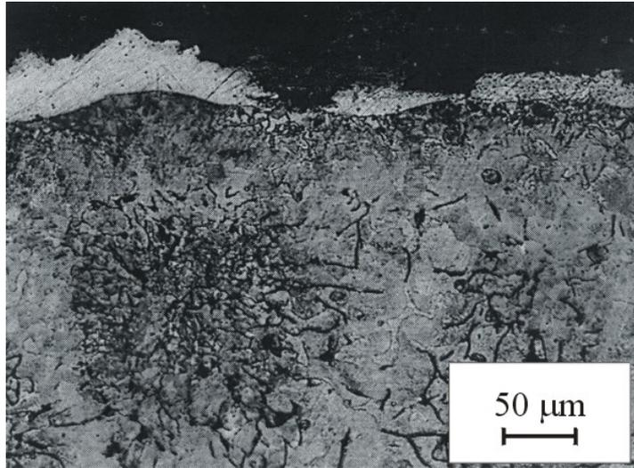
Fig. 3. Structure of casting's surface with one layer of VINAMUL 36/50 coating
