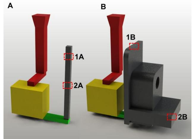
Fig. 1. The scheme of the gating system with experimental casts A and B; the places of cut of samples to the investigations of microstructure were marked dashed line
