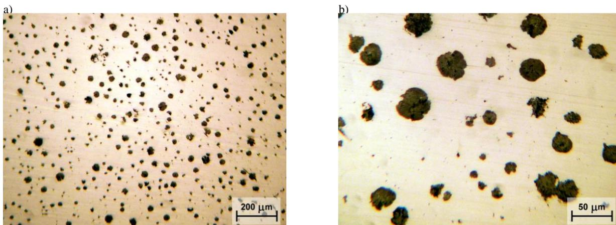
Fig. 5. The cast iron microstructure of the section 2B of the cast B a) magnification x100 b) magnification x400
