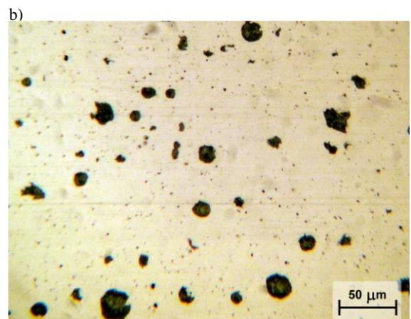
Fig. 4. The cast iron microstructure of the section 1B of the cast B a) magnification x100 b) magnification x400
