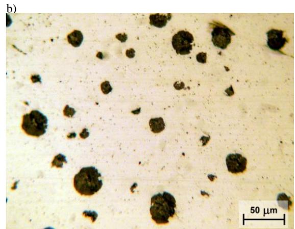
Rys. 3. The cast iron microstructure of the section 2A of the cast A a) magnification x100 b) magnification x400
