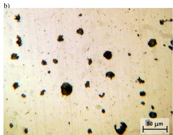
Fig. 2. The cast iron microstructure of the section 1A of the cast A a) magnification x100 b) magnification x400
