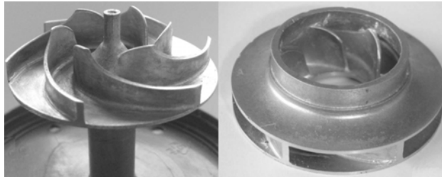
Rys. 4. Odlewy wirnika pompy. Wirnik otwarty i kompletny Fig. 4. Cast pump impellers. Opened impeller and closed impeller
