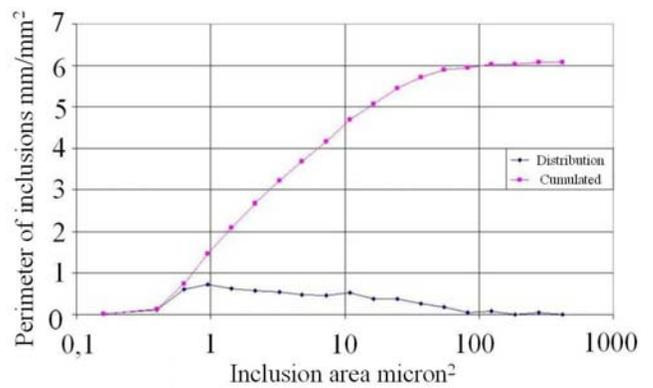
Fig. 6. Parameters describing inclusions – perimeter– non-filtered sample.
