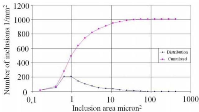
Fig. 4. Parameters describing inclusions – number– non-filtered sample.
