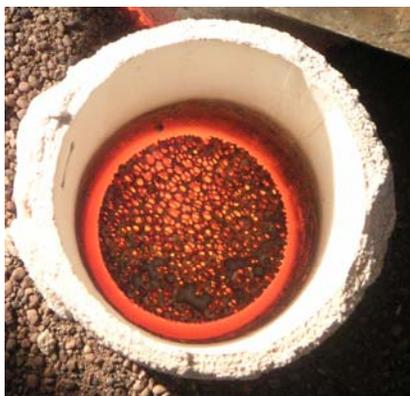
Fig. 1 Ceramic filter placed in mould –the appearance after metal flow.
