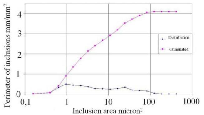
Fig. 7. Parameters describing inclusions – perimeter– filtered sample.
