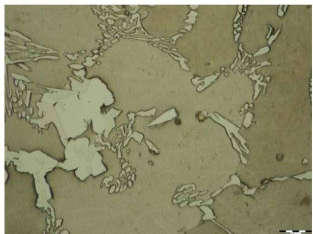
Fig.11. Microstructure of filtered sample - metallic matrix; polished section etched in LBI, .500x.
