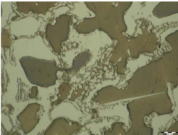
Fig.13. Microstructure of non-filtered sample - metallic matrix; polished section etched in LBI, 500x.
