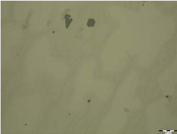
Fig.8. Microstructure of non-filtered sample. Unetched section; 500x.
