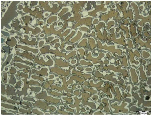
Fig.12. Microstructure of non-filtered sample - metallic matrix; polished section etched in LBI, 100x.
