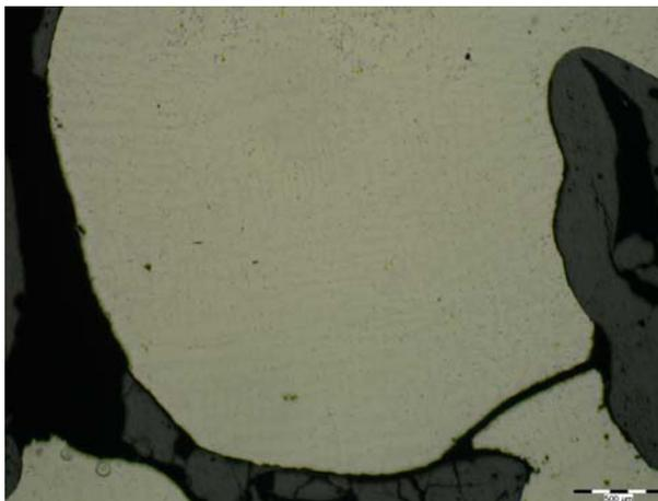
Fig.14. Cast metal/ceramic filter interface; unetched polished section, 25x.
