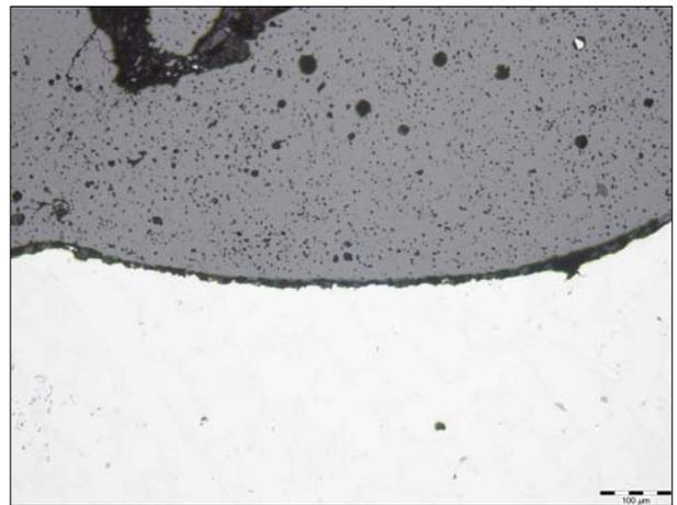
Fig.15. Cast metal/ceramic filter interface; unetched polished section; 100x.
