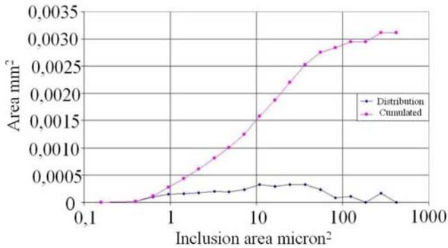
Fig. 2. Parameters describing inclusions – area– non-filtered sample.
