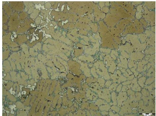
Fig.10. Microstructure of filtered sample - metallic matrix; polished section etched in LBI, .100x.
