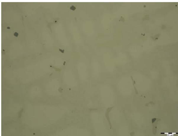
Fig.9. Microstructure of filtered sample. Unetched section; 500x.
