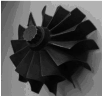
Fig.1. Aircraft impeller – high-alloy cast steel
