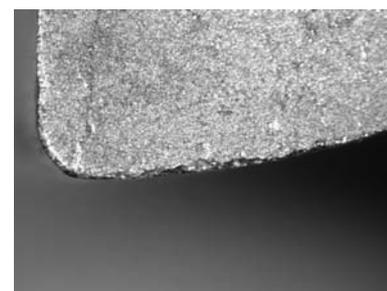
Fig. 8. Wall joint of the sintered powder sleeve (external shape  $\varnothing 26$ )
