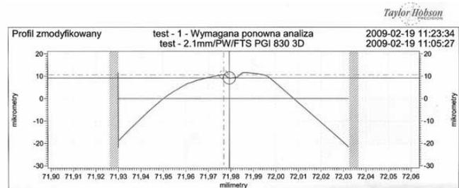
Fig.5. Wall joint of the sintered powder sleeve (external shape  $\phi 26$ )
