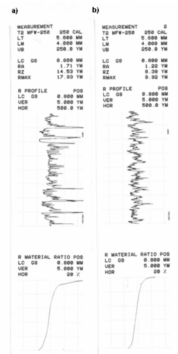
Fig. 6. Exemplary profilogram with the bearing ratio  $tp_{50}$  a) for sintered powder sleeve, b) for blade casting
