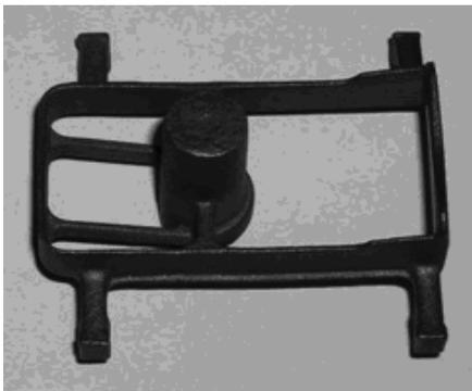
Fig.3. Frame with shank – alloy cast steel
