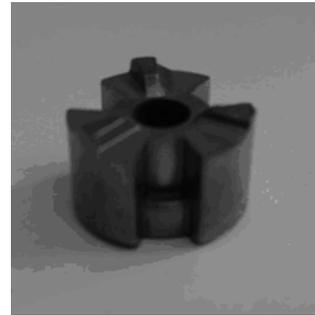
Fig.4. Indented sleeve – product made of sintered powders, Distaloy AB
