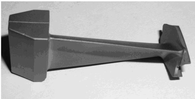
Fig.2. Aircraft blade – high-alloy cast steel. Thin wall casting in the middle part, thickness from 1.0 to 1.5 mm
