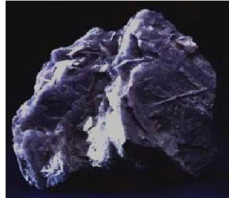
Fig. 3. Exterior grit NanoWin (NW) with nanocrystalline alumina sintered [4]
