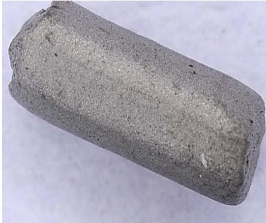
Fig. 1. General view of abrasive grain 76A of ordinary sintered alumina [2] In 1983, the same corporation conducted by sol-gel synthesis of the first alumina sintered submicrocrystalline, a trade name Cubitron (CB)
