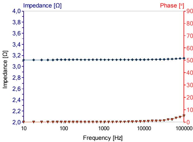
Fig. 2. Impedance spectra of graphite layer fabricated using paste P6 and fired at temperature 375 °C by 30 minutes
