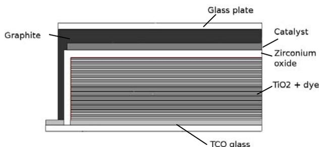
Fig. 1. The monolithic setup of DSSC cell
