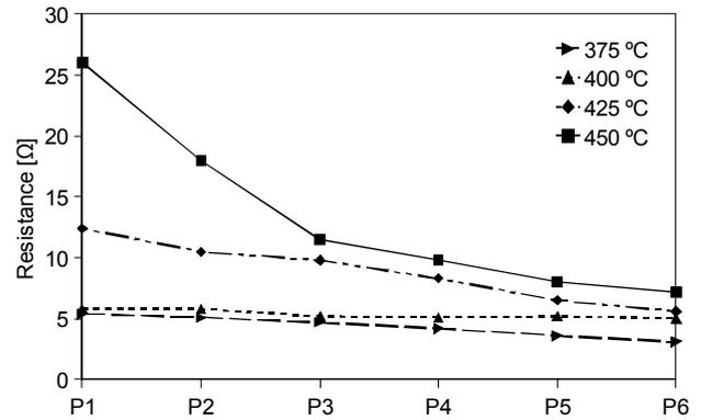
Fig. 3. Resistance of graphite layers vs. paste composition after different temperatures of heat treatment
