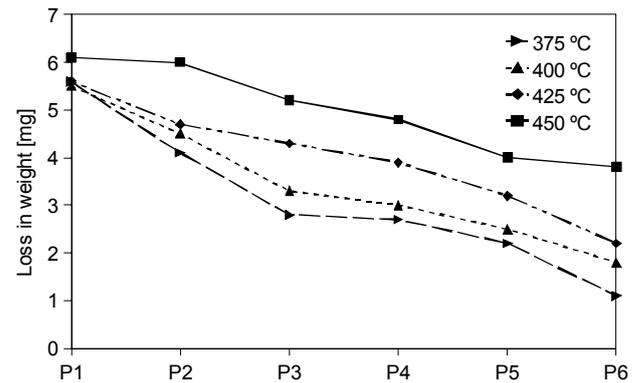
Fig. 4. Adhesive test results: loss in weight vs. paste composition
