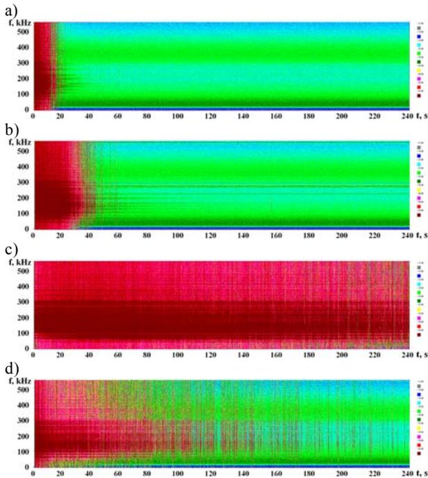
Fig. 1. Spectrograms of acoustic emission signals for the LH15SG steel after austempering at: a) 30 °C, b) 100 °C, c) 160 °C, d) 190 °C. The x-axis indicates the signal recording time (240 s), while the y-axis presents the recorded signal frequency in the linear scale of 0–600 kHz. The colours encode the chemical element value from the power spectral density of the recorded signal in a 9-grade scale. The lowest signal power is marked dark-blue, while the highest is dark-red
