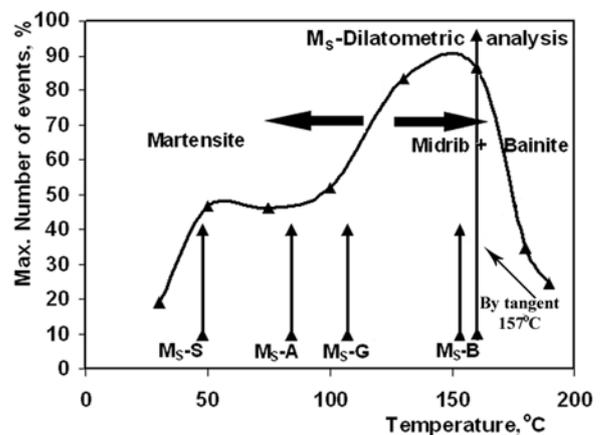
Fig. 2. A distribution of the sum of acoustic event numbers during austempering. In the y-axis, 100% corresponds to  $5 \times 10^7$  events. In the figure, the  $M_S$  calculation results with the use of Steven's ( $M_S$ -S), Andrews' ( $M_S$ -A), Grange's ( $M_S$ -G), Bohemen's ( $M_S$ -B) [14-17] equations are also presented
