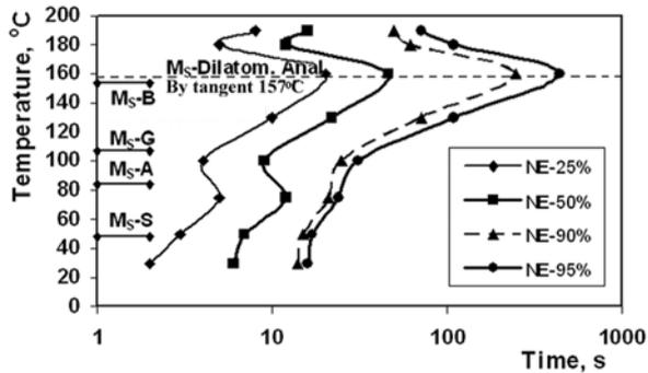
Fig. 3. The time-temperature-acoustic emission (TTEA) curve during austempering together with the experimental calculation results of the  $M_s$  temperature
