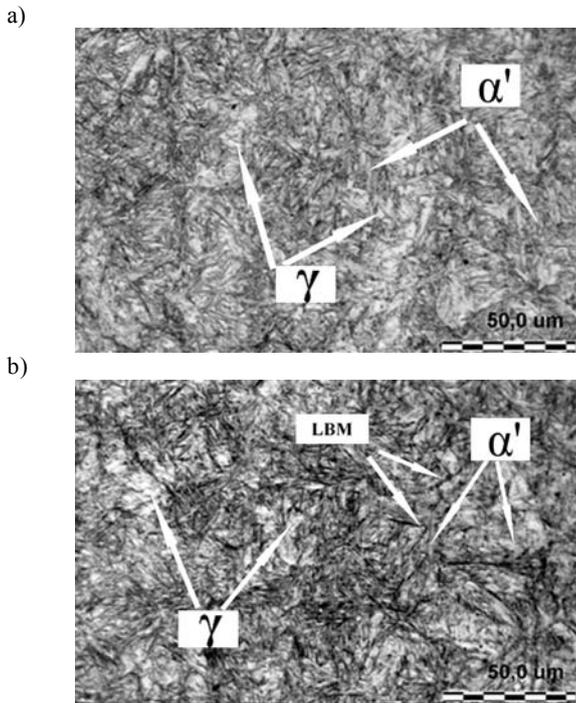
Fig. 4. Optical microscopic pictures of the specimens after isothermal transformation with holding time of 1450 s at different temperatures: a) 100°C, b) 160°C, etching with Nital reagent, holding time: 1450 s. The symbols  $\alpha'$ ,  $\gamma$ , LBM stand for martensite, retained austenite and bainite, respectively
