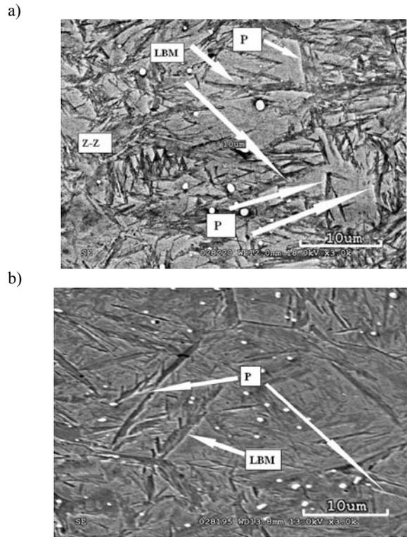
Fig. 5. Scanning electron micrographs of specimens isothermally treated with the holding time of 1450 s at temperatures: a) 160°C, b) 190°C; etched with a Nital reagent. The dark plates are lower bainite with midrib LBM and light places around the plates are untransformed retained austenite P. In the micrograph 5a), plate martensite with a characteristic morphology Z-Z is seen
