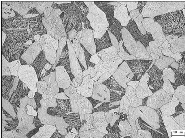
Fig. 4. Optical photomicrograph of ferrite and bainite in the A steel, after etching 5% HNO<sub>3</sub>, 200x
