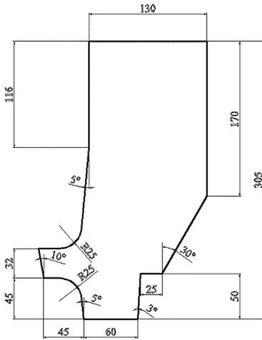
Fig. 3. Geometry of the casting with raiser (size in millimeters)
