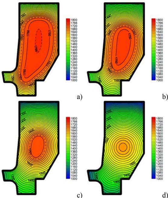
Fig. 6. Temperature of the casting according to high cooling rate on the top boundary after a) 500 [s], b) 750 [s], c) 1000[s], d) 1175 [s]
