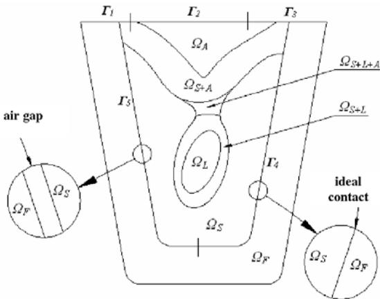
Fig. 1. Mould and casting consisted of regions filled with mixture of the solid, liquid and gas
