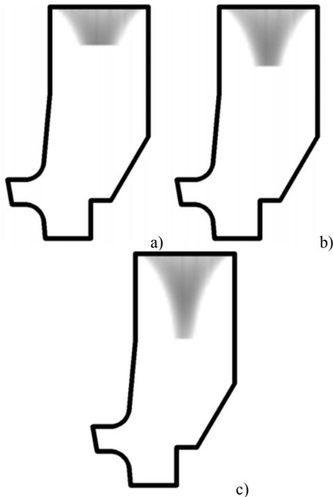
Fig. 7. Shape of the shrinkage cavity according to high cooling rate on the top boundary after a) 500 [s], b) 750 [s], c) 1000[s]
