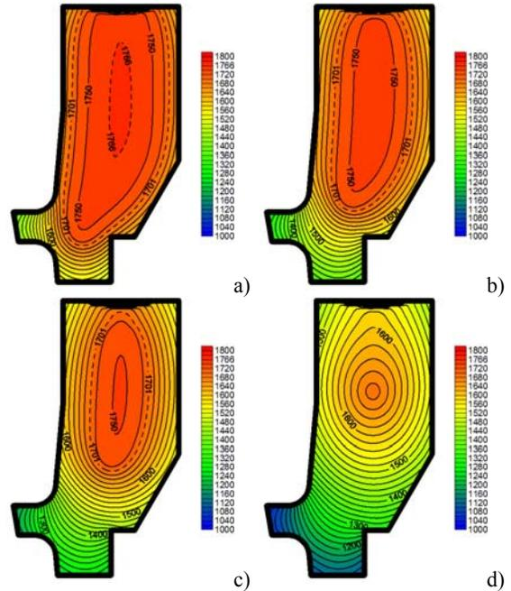
Fig. 4. Temperature of the casting according to low cooling rate on the top boundary after a) 500 [s], b) 750 [s], c) 1000[s], d) 1350 [s]
