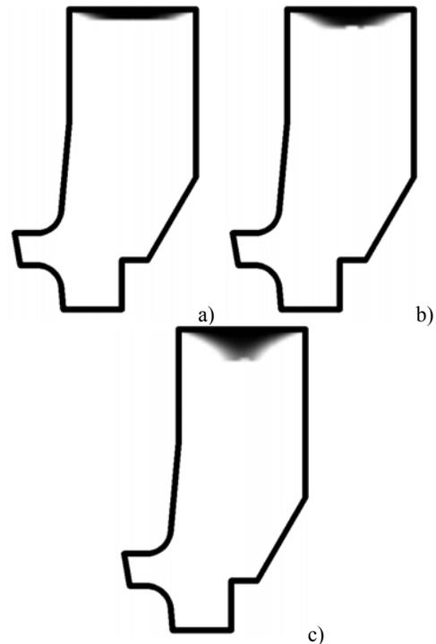
Fig. 5. Shape of the shrinkage cavity according to low cooling rate on the top boundary after a) 500 [s], b) 750 [s], c) 1000[s]
