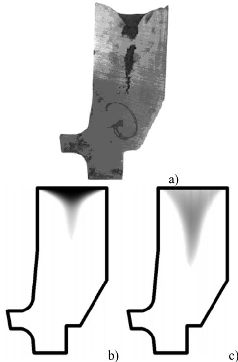
Fig. 8. Shape and localization of the shrinkage cavity a) real defect, b) simulation with low cooling rate on the top boundary, c) simulation with high cooling rate on the top boundary
