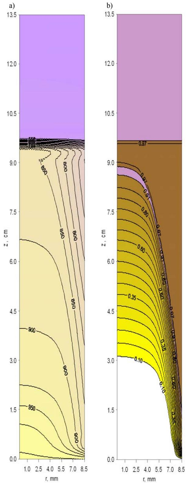
Fig. 3. Temperature field (a) and solid phase fraction (b) after stopping of the molten metal flow (simplified model)
