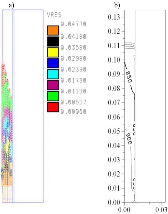
Fig. 2. Velocity vectors (a) and temperature field (b) after stopping of the molten metal flow (general model)
