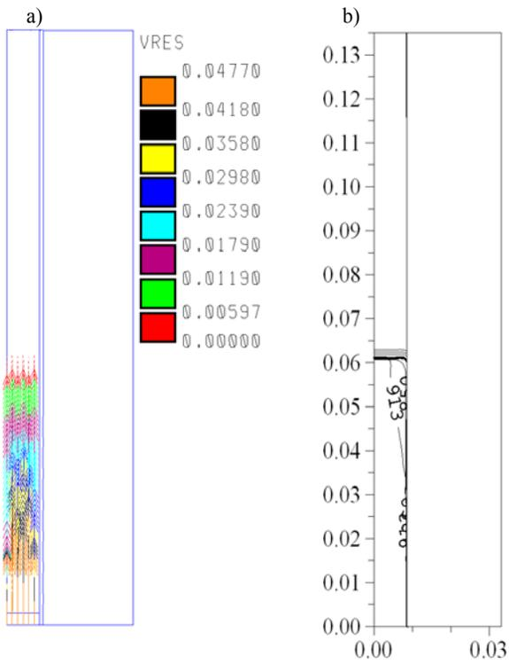
Fig. 1. Velocity vectors (a) and temperature field (b) during the mould cavity filling of the vertical fluidity test (general model)
