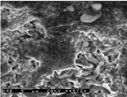
Fig. 2. SEM of wear surface of composite material with 10% of Al<sub>2</sub>O<sub>3</sub> after wear distance of 8.5 km
