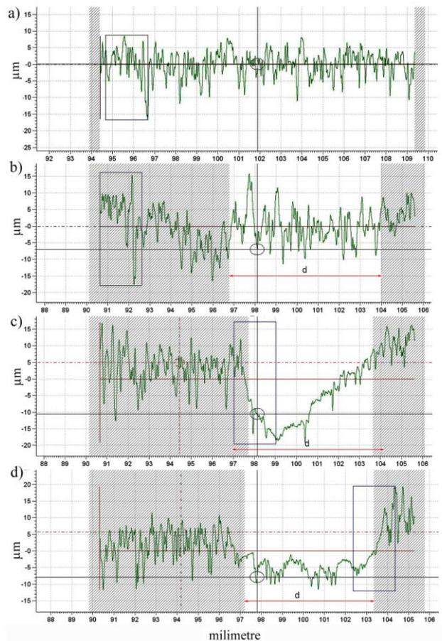
Fig. 3. The roughness profiles of discs from cast-iron after wear distance of 8.5 km, a) for clear disk from cast iron b) after wear against not reinforced CuZn38Al2Mn1Fe brass c) after wear against composite material brass – 10 vol. % of Saffil d) after wear against brass -20 vol.% of Saffil
