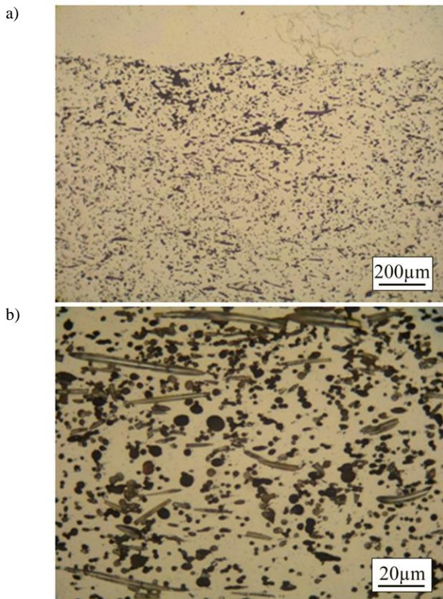
Fig. 1. Microstructure of the CuZn38Al2Mn1Fe brass with with SAFFIL fibres a) border zone of composite material containing 10 vol. % of Saffil fibres b) material containing 20 vol. % of fibres
