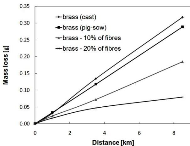
Fig. 4. Change of mass loss as the function of the wear distance
