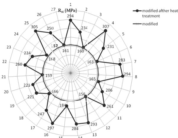
Fig. 6. Change of the  $R_m$  tensile strength of the EN AB-AlSi17Cu1Ni1Mg alloy for individual configurations of the testing plan
