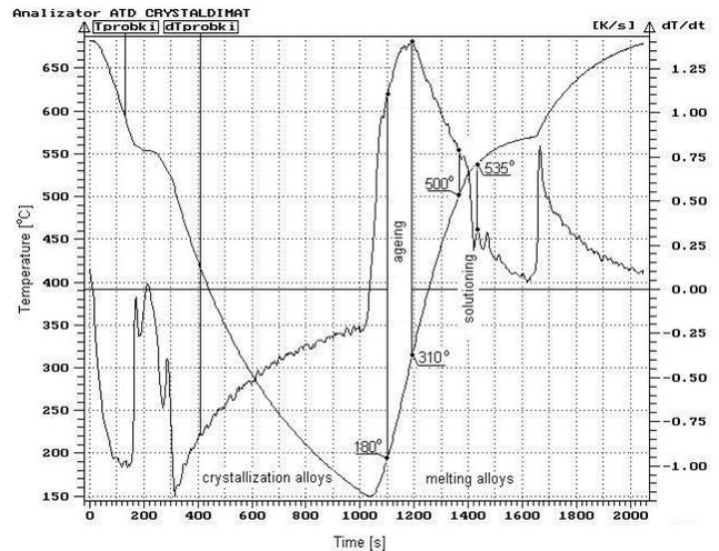
Fig. 2. Curves from the ATD method for the refined and modified EN AB- AlSi12CuNiMg alloy
