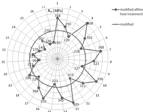
Fig. 4. Change of the  $R_m$  tensile strength of the EN AB-AlSi9Cu3(Fe) alloy for individual configurations of the testing plan
