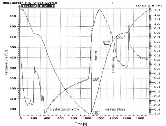
Fig. 3. Curves from the ATD method for the refined and modified EN AB- AlSi17Cu1Ni1Mg alloy
