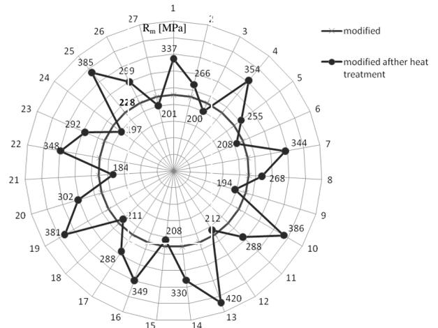
Fig. 5. Change of the  $R_m$  tensile strength of the EN AB-AlSi12CuNiMg alloy for individual configurations of the testing plan
