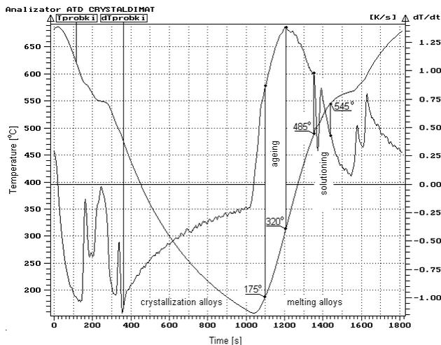
Fig. 1. Curves from the ATD method for the EN AB-AlSi9Cu3(Fe) alloy
