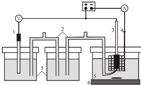
Fig. 1. Diagram of the measuring system for electrochemical dissolution; 1 – calomel electrode, 2 – salt-bridge, 3 – sample, 4 – platinum electrode, 5 – electrolytes, 6 – electromagnetic stirrer [9]
