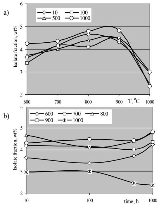
Fig. 4. Weight percent fraction of isolates vs a) temperature and b) time of cast steel annealing
