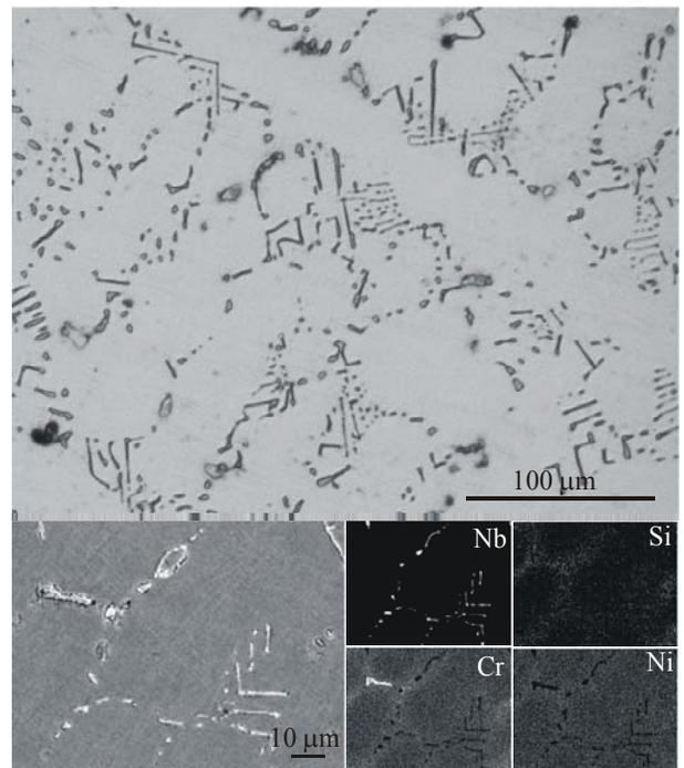
Fig. 2. Microstructure of alloy in as-cast state and distribution of alloy chemical constituents
