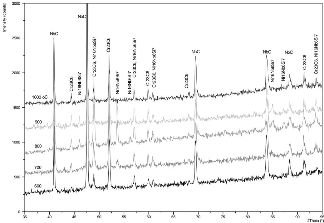
Fig. 3. X-ray diffraction spectra of isolates after 1000 h annealing at temperature 600, 700, 800, 900 i 1000°C
