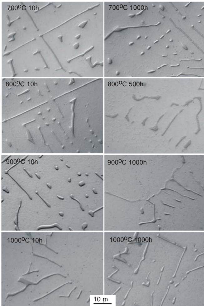
Fig. 5. Microstructure of annealed cast-steel, Nomarski Contrast
