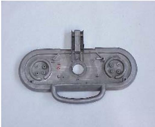
Fig. 3. Non anodized element made from the AC-AlSi12 aluminium alloy, produced by the Pressure Cast method
