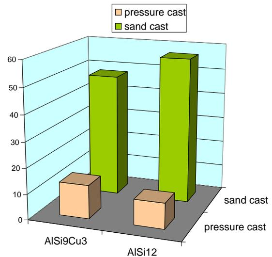
Fig. 6. Results of the anodic layer thickness measurement
