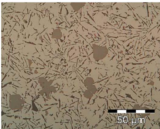
Fig. 11. Microstructure of the AlSi12 alloy, high pressure cast
