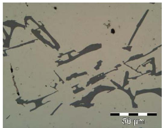
Fig. 10. Microstructure of the AlSi12 alloy, sand cast
