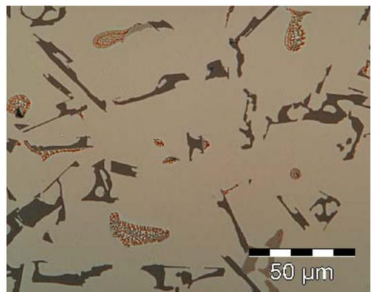
Fig. 12. Microstructure of the AlSi9Cu3 alloy, sand cast
