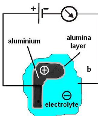
Fig. 1. Scheme of the anodization process including the anodized part, electrolyte, power supply and the alumina surface layer.
