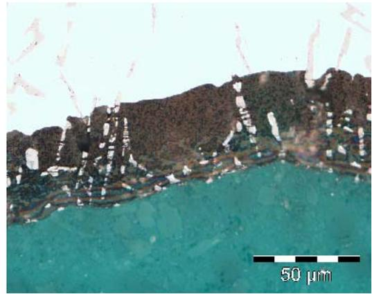
Fig. 8. Anodic alumina layer generated on the AlSi12 alloy, sand cast
