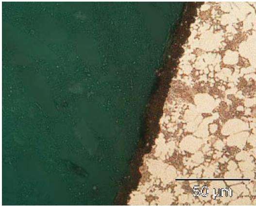
Fig. 7. Anodic alumina layer generated on the AlSi9Cu3 alloy, high pressure cast
