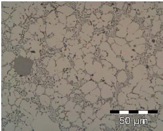
Fig. 9. Microstructure of the AlSi9Cu3 alloy, high pressure cast
