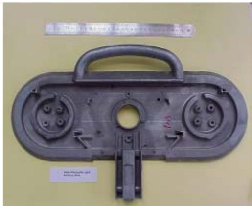
Fig. 4. Anodized element made from the AC-AlSi9Cu3 aluminium alloy, produced by the Pressure Cast method
