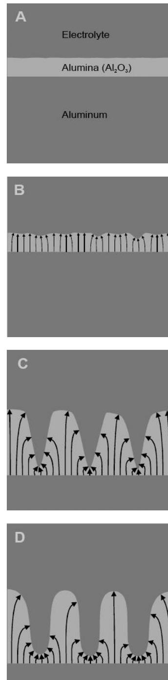
Fig. 2. Stages in the development of the alumina surface layer, a) barrier layer development, b) growth of small inhomogenities, c) continuously grow of pores, d) stabilization of the interpore distances (JPK Instruments AG, 2003).
