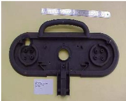
Fig. 5. Overanodized element made from the AC-AlSi9Cu3 aluminium alloy, produced by the Pressure Cast method
