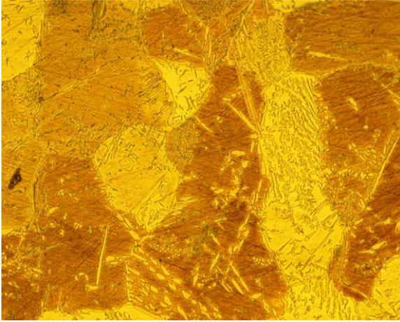
Fig. 4c. CuZn44Te2; Magnification 100x
