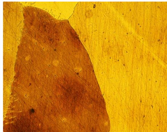
Fig. 4b. CuZn44Te1.5; Magnification 100x
