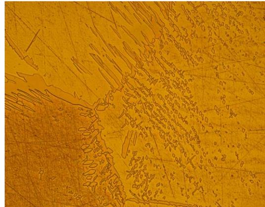
Fig. 1c. CuZn44Co0.5; Magnification 500x
