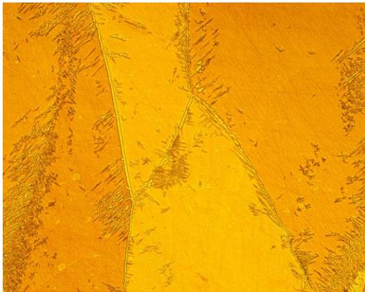
Fig. 2a. CuZn44Ni0.5; Magnification 100x
