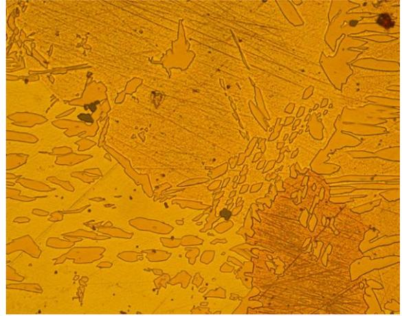
Fig. 4d. CuZn44Te2; Magnification 500x
