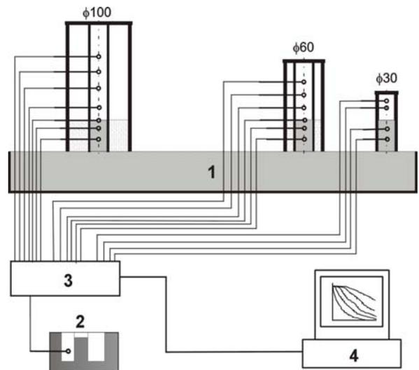
Fig. 3. Scheme of test stand: 1 - set of testers DTA-K 3, 2 - tester DTA-C, 3 - transducer A/C, 4 - computer PC
