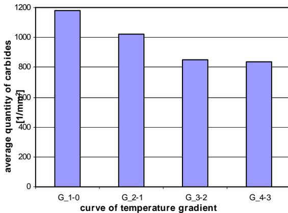
Fig. 7. The average the quantity of carbides in function of curve the temperature gradient on section of casting  $\phi 100$
