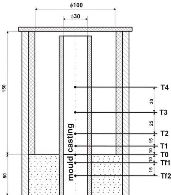
Fig. 1. The construction of tester  $\phi 100$  mm
