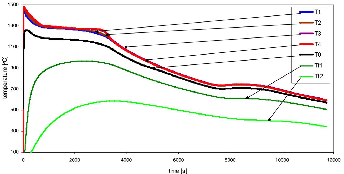
Fig. 4. Curves cooling in tester cast and form  $\phi 100$
