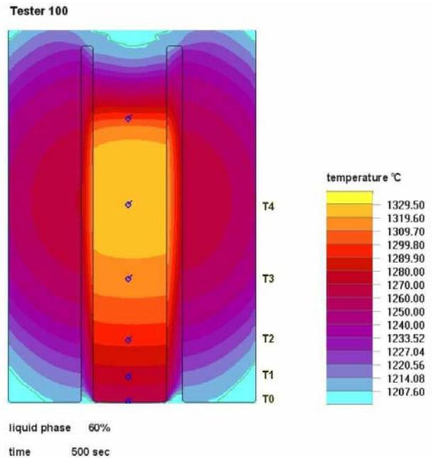
Fig. 2. Simulation cooling of tester  $\phi 100$  mm
