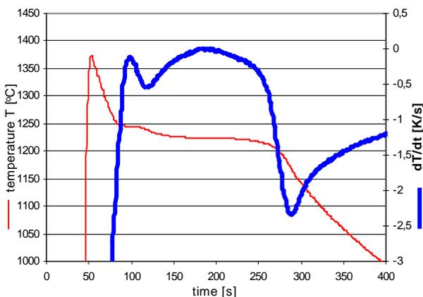
Fig. 5. Curves DTA-C studied chromium cast iron
