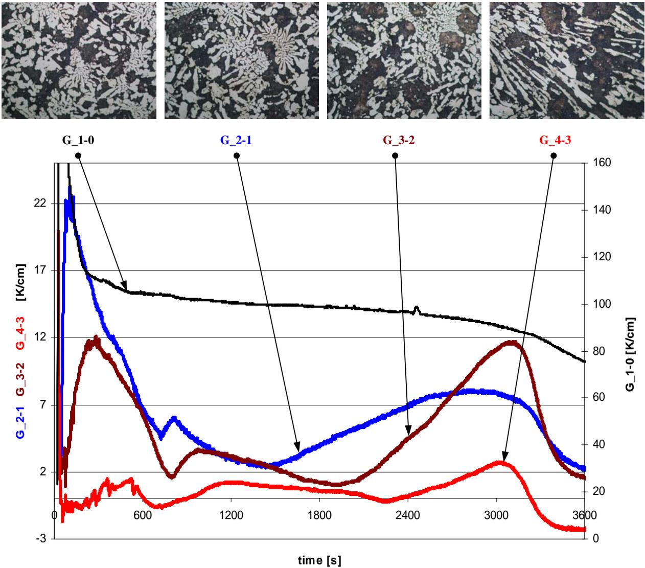
Fig. 6. Curves temperature gradient in range of primary crystallization of chromium cast iron on section of casting the  $\phi 100$  and answering them structures with clear carbide phase (x200)
