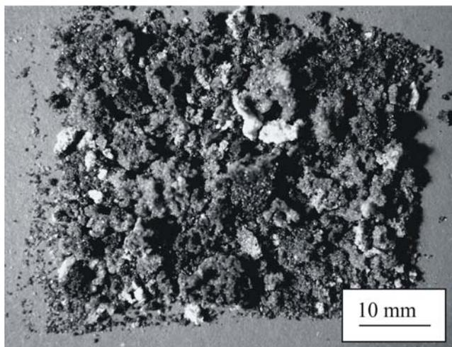
Fig. 5. Waste shell moulds and cores after burning in microwave chamber with intensifying additive
