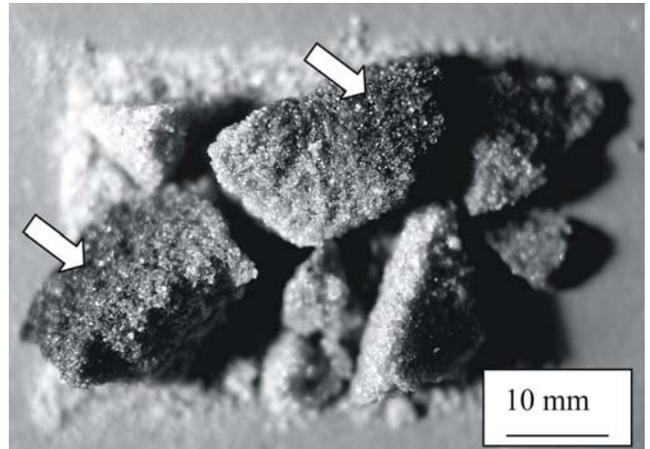
Fig. 2. Waste shell moulds and cores after burning in microwave chamber (arrows indicate partially burnt areas)
