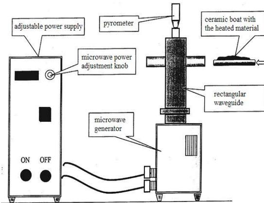
Fig. 1. Test stand for incineration using microwave heating
