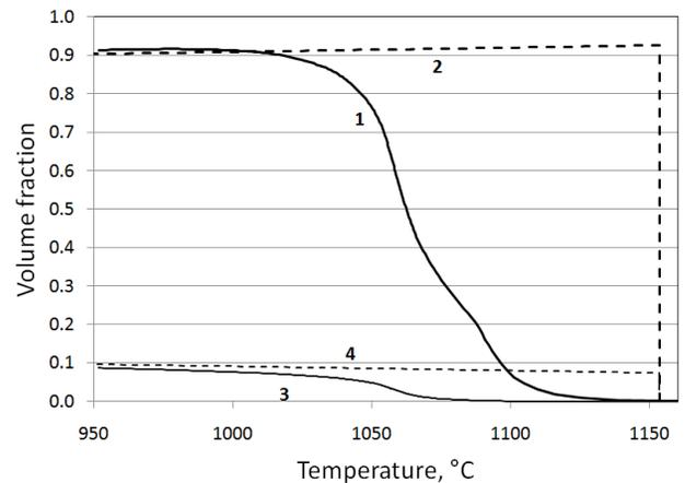
Fig. 1. Austenite (1,2) and graphite (3,4) volume fraction as a function of temperature: 1, 3) CA modeling; 2, 4) thermodynamic equilibrium (obtained by ThermoCalc software)
