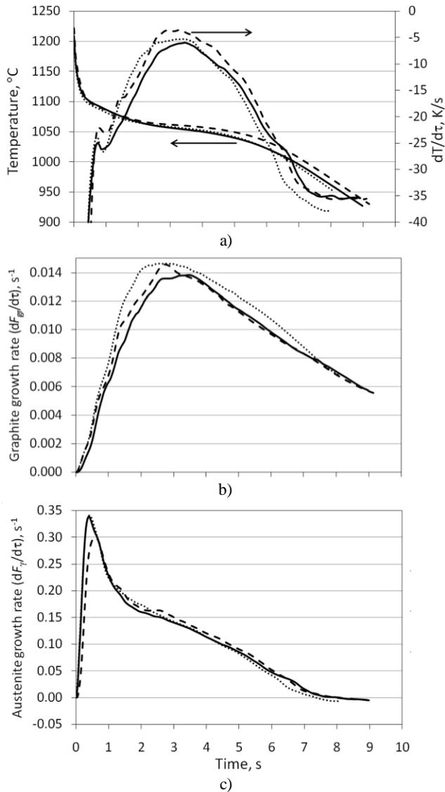
Fig. 2. Cooling curves and cooling rates of DI (a), and graphite (b) and austenite (c) growth rate: solid lines – hypo-eutectic DI, dotted lines – eutectic DI, and dashed lines – hyper-eutectic DI
