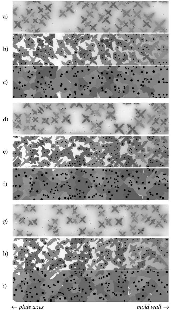
Fig. 3. Structure formation of the hypo-eutectic (a-c), eutectic (d-f) and hyper-eutectic (g-i) DI during the solidification into 2 mm wall (simulation results); solidification time: (a,d,g) – 0.7 s; (b,d,h) – 3.2 s; (c,f,i) – 7.2 s
