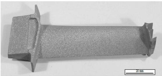
Fig. 2. Macrostructure of blade made of IN-100 – test 2
