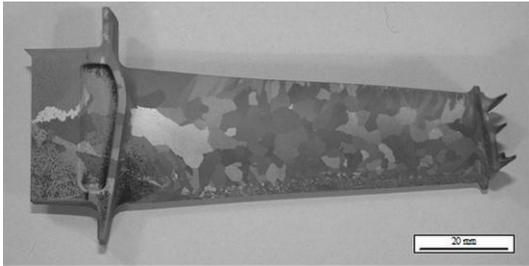
Fig. 1. Macrostructure of blade made of IN-100 – test 1
