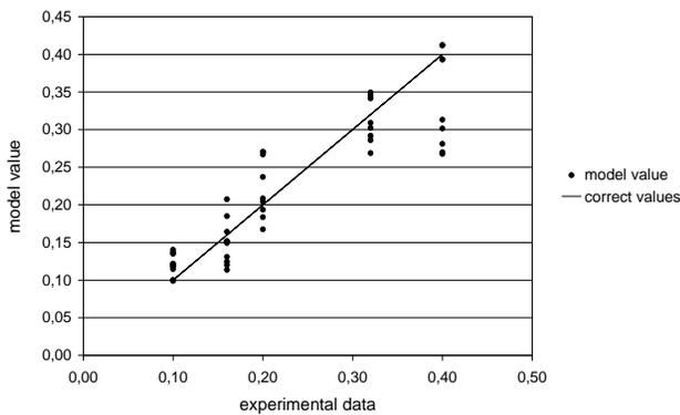
Fig. 7. Comparison of the distribution of data generated by the network and the experimental data, input data: permeability, output data: sand grain size, the network model RBF 1-12-1
