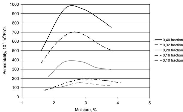
Fig. 2. The influence of water content on permeability, for the moulding sands with different grain size
