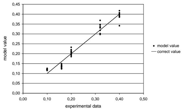
Fig. 9. Comparison of the distribution of data generated by the network and the experimental data, input data: permeability, compactability, compressive strength, output data: sand grain size, the network model MLP 3-3-1
