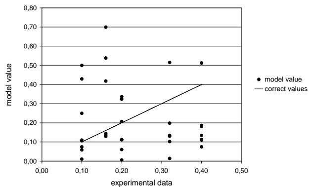
Fig. 5. Comparison of the distribution of data generated by the network and the experimental data, input data: compressive strength, output data: sand grain size, the network model: RBF 1-17-1
