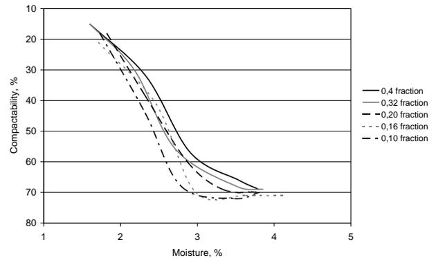
Fig. 3. The influence of water content on compactibility, for the moulding sands with different grain size
