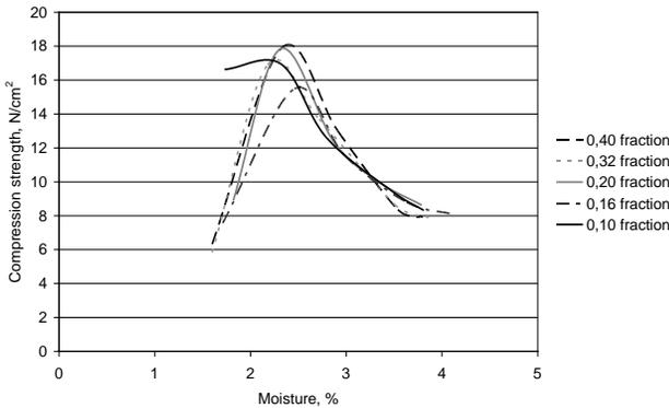
Fig. 1. The influence of water content on compressive strength  $R_c^W$ , for the moulding sands with different grain size
