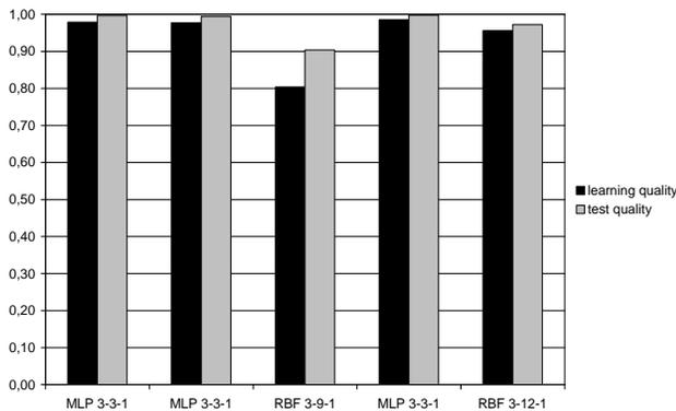
Fig. 10. Learning and test quality comparison, input data: permeability, compactability, compressive strength
