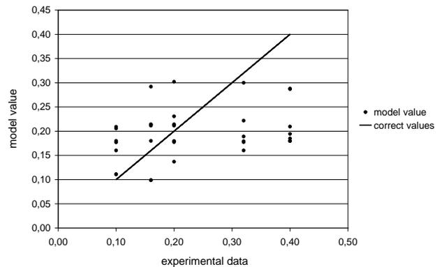
Fig. 4. Comparison of the distribution of data generated by the network and the experimental data, input data: compactibility, output data: sand grain size, the network model: RBF 1-9-1
