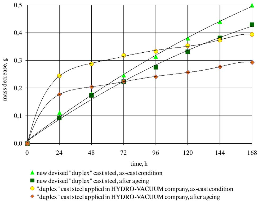
Fig. 5. Mass decrease in water solution of 15% HCl of tested grades of cast steel as-cast and after ageing
