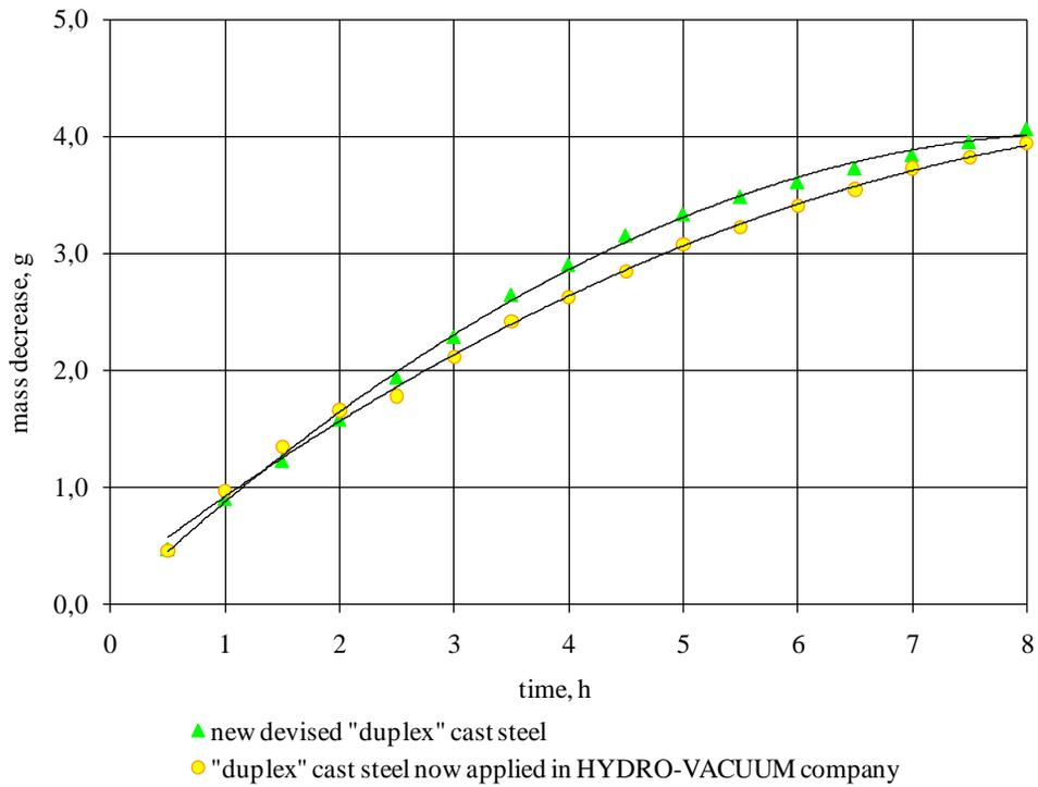
Fig. 4. Abrasive wear of „duplex” cast steel now applied in HYDRO-VACUUM company and the new
