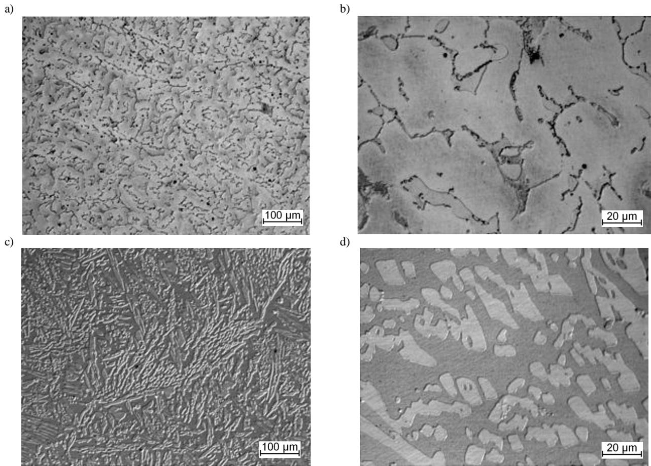
Fig. 2 (a-d). The microstructure of „duplex” cast steel after solution heat treatment, now applied (a, b) and new devised (c, d)
