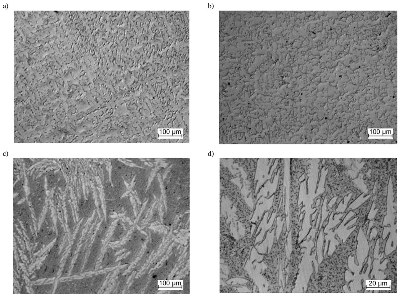
Fig. 1 (a-d). The microstructure of „duplex” cast steel now applied (a, b) and new (c, d)
