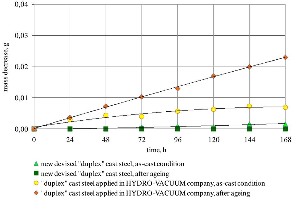
Fig. 6. Mass decrease in water solution of 15% H<sub>2</sub>SO<sub>4</sub> of tested grades of cast steel as-cast and after ageing
