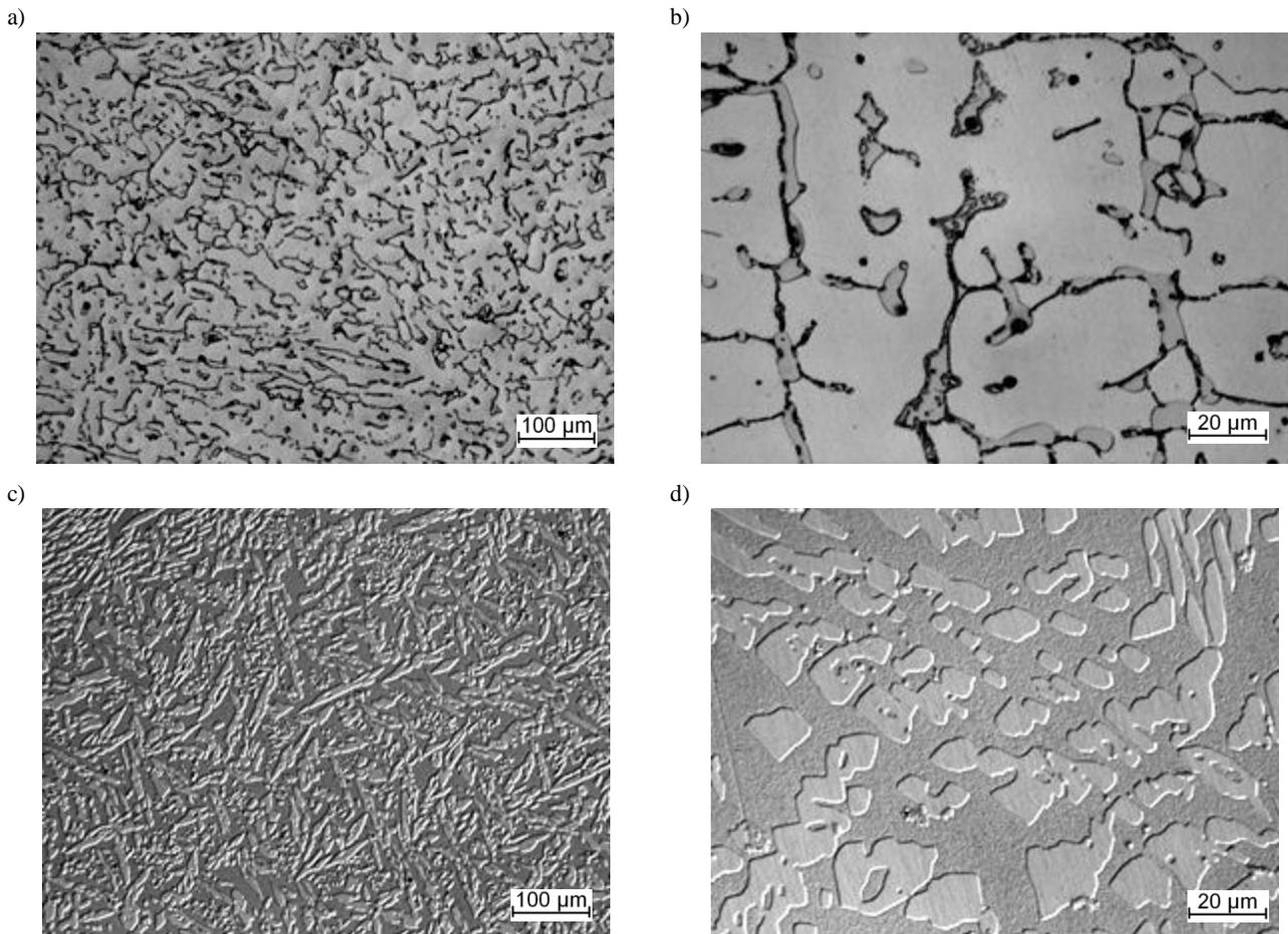
Fig. 3 (a÷d). The microstructure of „duplex” cast steel after ageing, now applied (a, b) and new (c, d)
