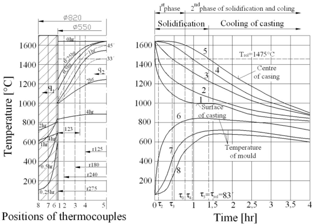
Fig. 5 a, b. Temperature field in steel cylinder casting with diameter 550 mm and in a metallic mould
