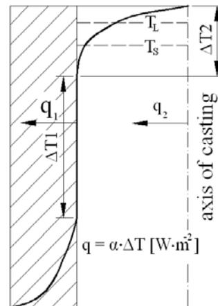
Fig. 4. Schematic drawing of thermal gradients and heat flow in a casting and a mould
