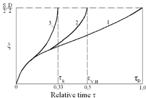
Fig. 2. Characteristic curves for isosolidus progression of basic shape castings
