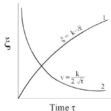
Fig. 3. The thickness of solidified layer of metal and solidification velocity
