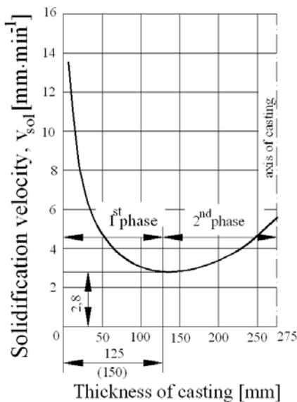
Fig. 6. Solidification velocity in cross section of steel cylinder with diameter 550 mm
