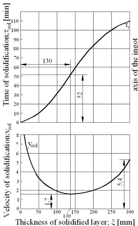
Fig. 8. The solidification velocity in cross section of steel ingot 600 x 600 mm, weight 4,8 t
