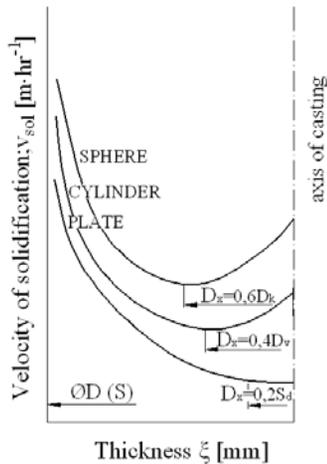
Fig. 1. Comparison of calculated solidification rate in cross section of basic shape castings
