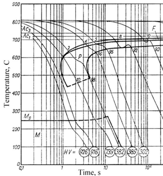
Fig. 2. Diagram CCT for steel C80U [9]
