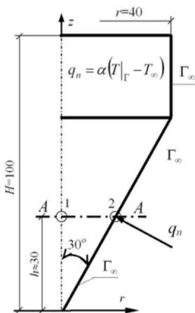
Fig. 7. Form and dimensions of the hardening object
