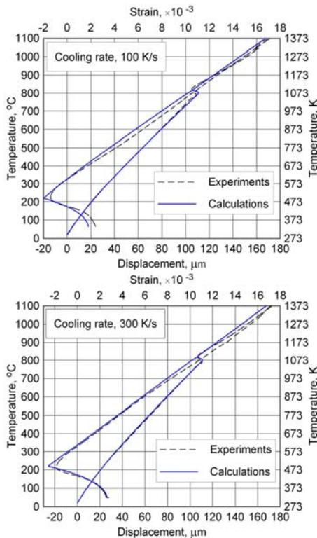
Fig. 5. Experimental and simulating dilatometric curves
