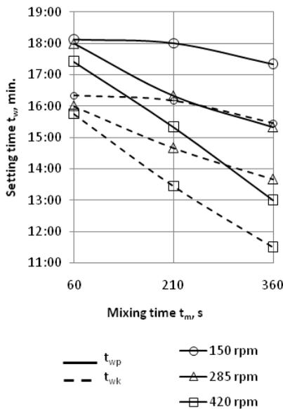
Fig. 3. The dependence between setting time of gypsum plaster  $t_w$  and mixing time  $t_m$
