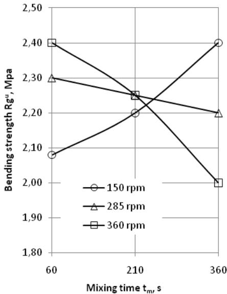
Fig. 5. The dependence between the bending strength of set plaster  $R_g^u$  and mixing time  $t_m$
