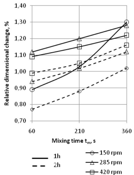
Fig. 4. The dependence between relative dimensional change of set gypsum plaster and mixing time  $t_m$
