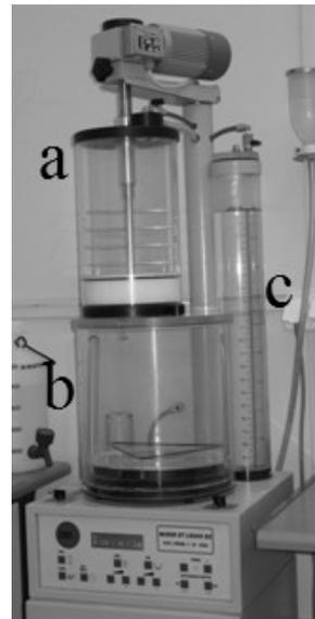
Fig. 1. Vacuum mixer St. LOUIS 82 B/P: a – vacuum chamber with frame mixing arm, b – casting moulds chamber, c- distilled water feeder
