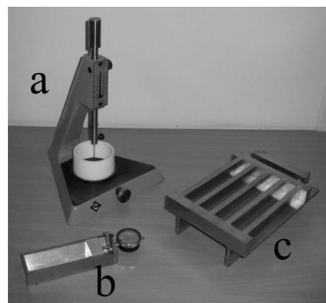
Fig. 2. Test stand for determination of technological properties of gypsum plaster: a – Vicat apparatus with measuring ring, b – form for linear dimensional changes determination of set plaster, c – experimental shape for lengthwise samples
