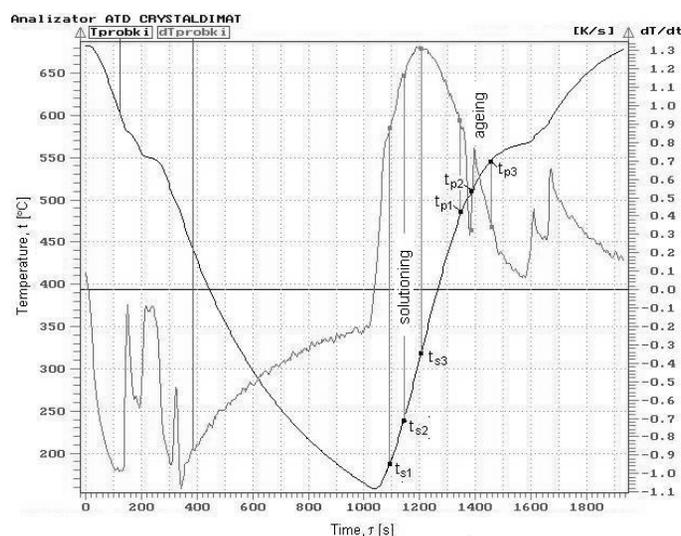
Fig. 1. Curves of the ATD method for refined and modified EN AC- $\text{AlSi9Cu3(Fe)}$  alloy
