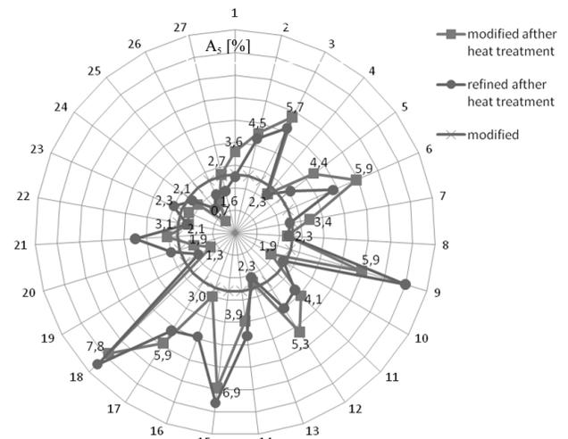
Fig. 3. Change of  $A_5$  elongation of the investigated alloy for individual configurations of the testing plan
