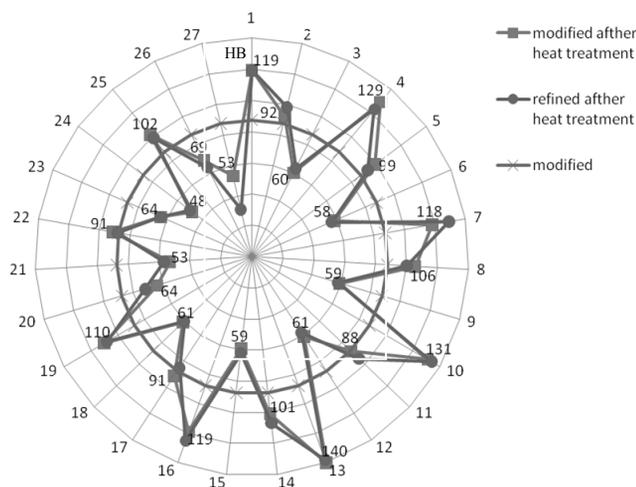
Fig. 4. Change of HB hardness of the investigated alloy for individual configurations of the testing plan
