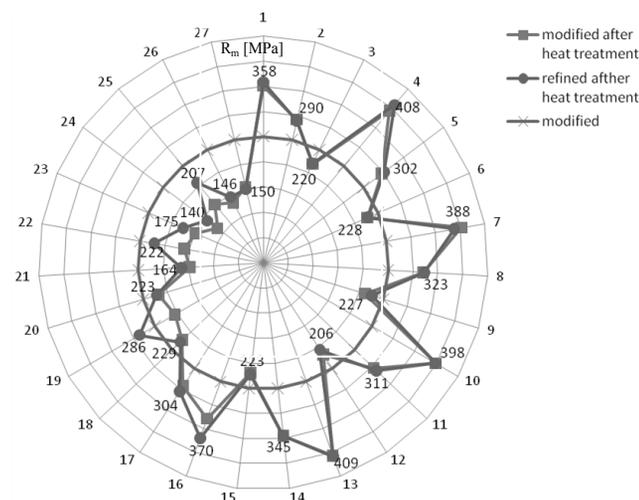
Fig. 2. Change of  $R_m$  tensile strength of the investigated alloy for individual configurations of the testing plan
